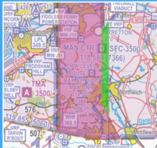
Figure 4 Visual depiction in green shading of extended areas of Class G airspace on VFR chart
