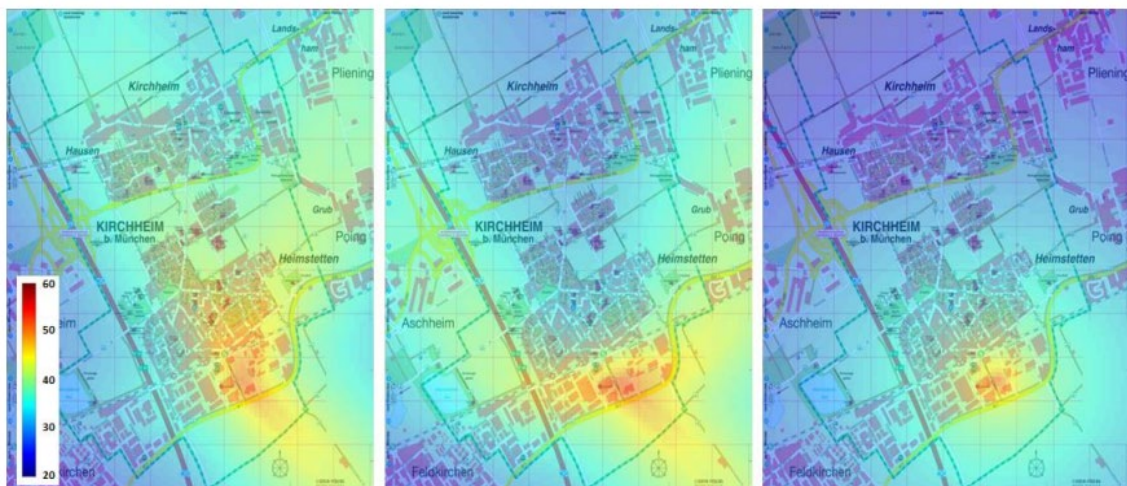
Figure 2: A-weighted L_{den} noise maps for the town area, showing the L_{den} for a) the baseline scenario ( 6^\circ slope), b) the optimised baseline and c) the steep approach and climb.
