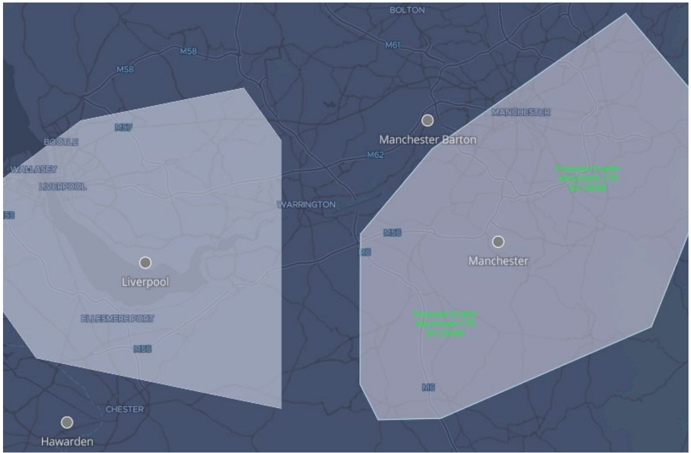
Figure 6 Proposed design of Manchester and Liverpool CTRs showing Class G airspace between them
