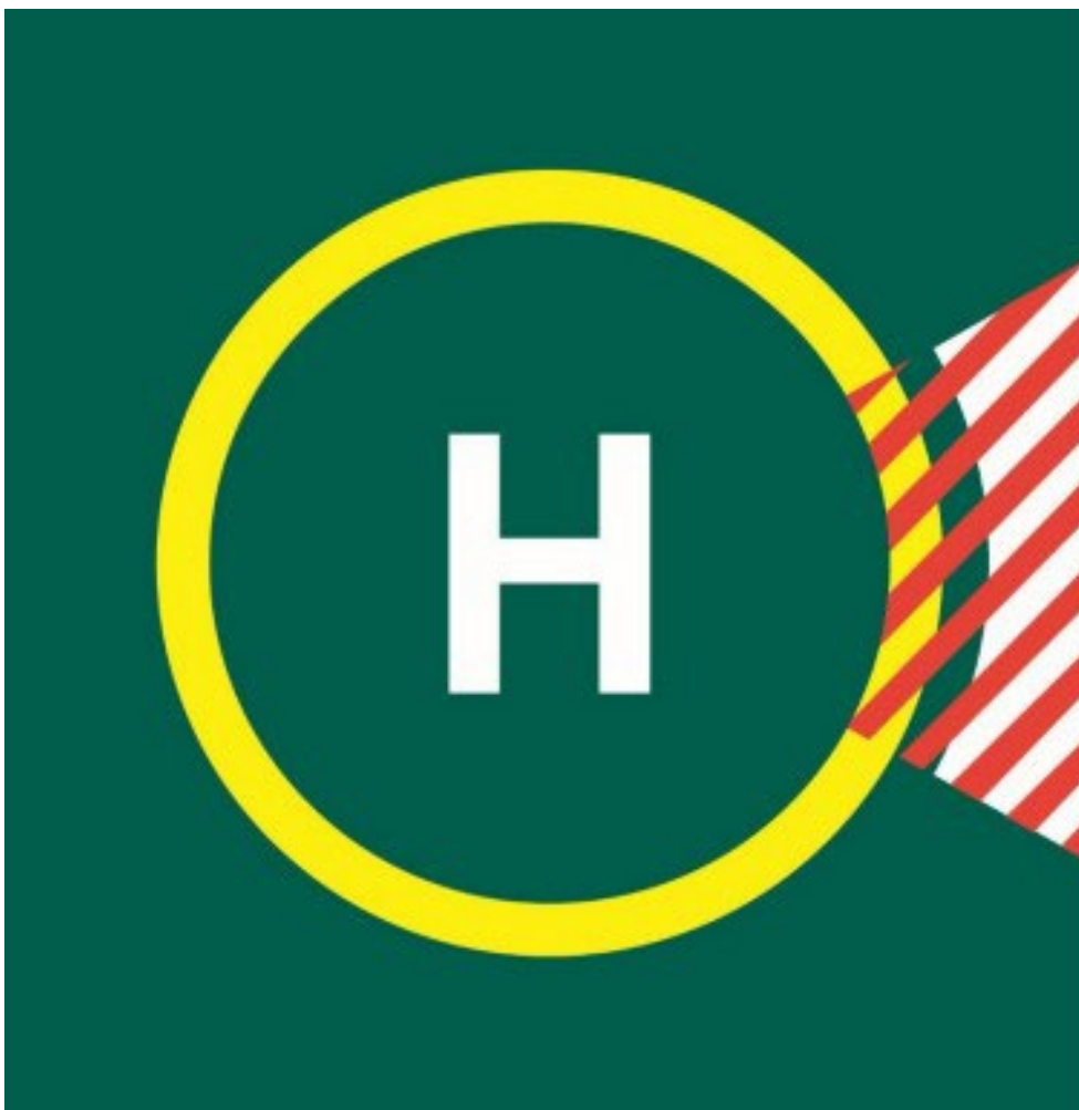
Figure 4-10: Example of prohibited landing heading marking
