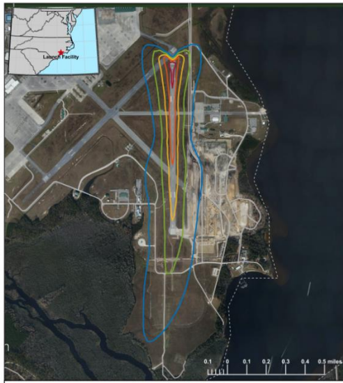
EXAMPLE DNL CONTOURS FOR A HORIZONTAL LAUNCH VEHICLE DNL Contours Map Features 65 dBA 70 dBA 75 dBA 80 dBA 85 dBA County Boundaries Roads
