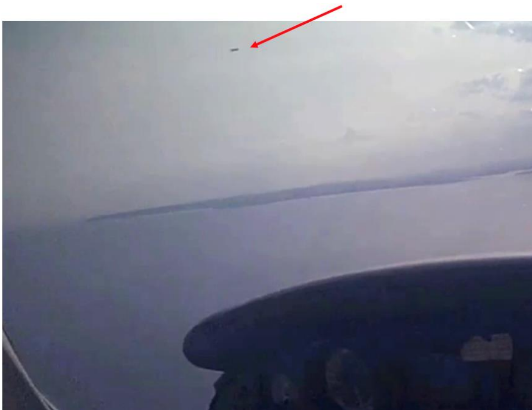
Figure 27 – Image from the eye-tracker scene camera showing the visual conditions. Target aircraft B is arrowed, and about to pass to the left at about 300-400m range (eye-tracker symbol removed). The eye tracker scene camera offers a misleading impression that the target is distant.
