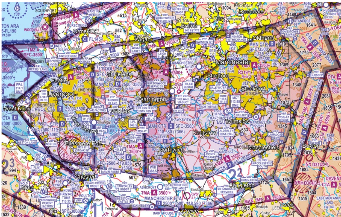
Figure 2 Screenshot of VFR 1:500,000 map (Edition 46: 22 April 2023) showing the location of the MLLR (pink north-south corridor in image centre)
