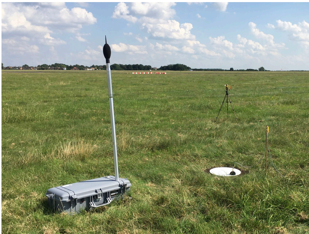
Figure C2 IGP and 1.2 m microphone installation at Cranfield Airport
