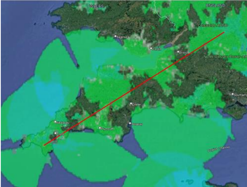
FIGURE 16 SURVEILLANCE COVERAGE AT 400 FT – DUAL BAND ADS-B RECEIVERS COLLOCATED WITH THE EXISTING RADARS
