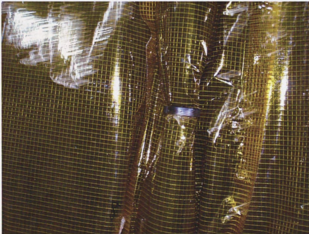
Figure 32 Test D2-1 Plastic Over Frame Clips on a 14" pitch
