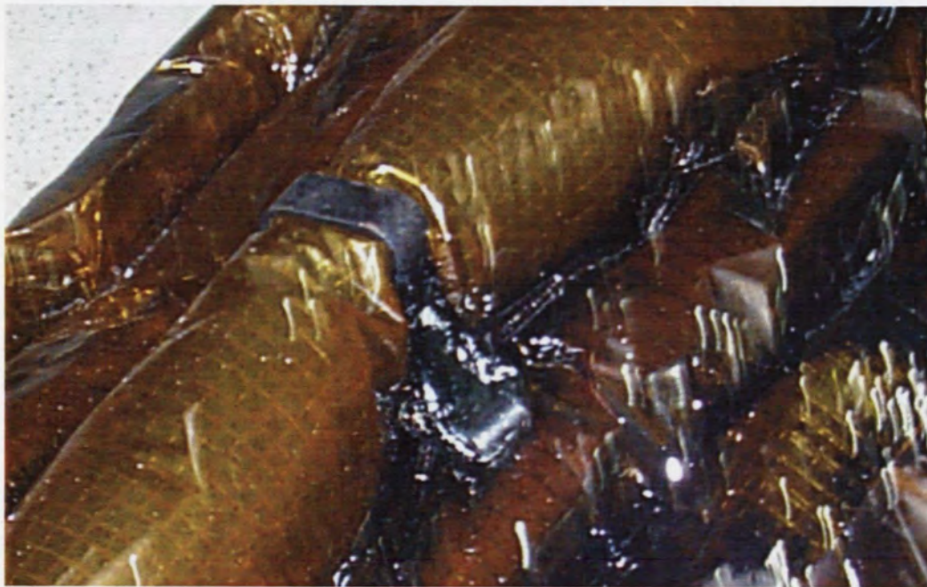
Figure 34 Test D2-3 Close up of Plastic Over Frame Clips after Testing
