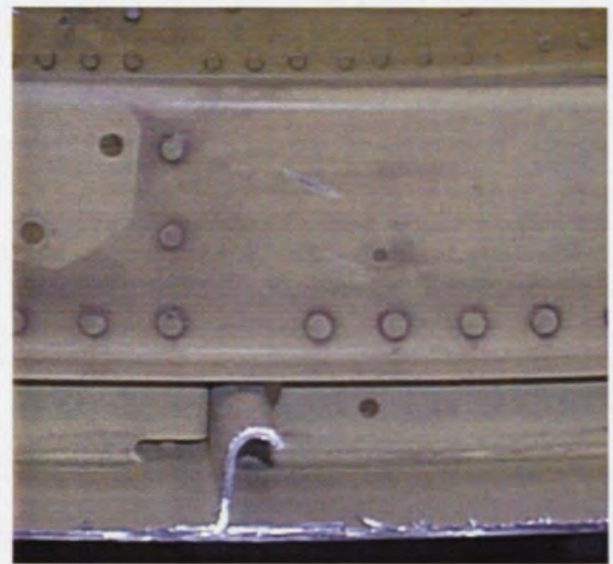
Figure 11 Frame and Stringer Details on Actual Aircraft panel
