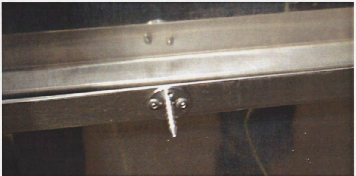
Figure 43 Test D5-1 Close Up of Aluminium Stringer Pin attached to Stringer
