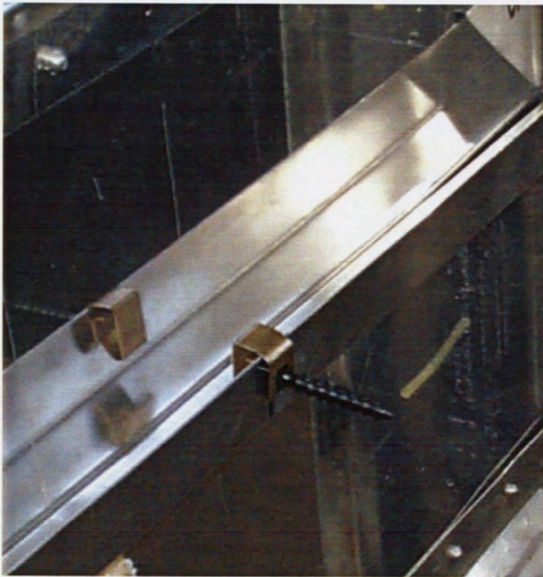
Figure 16 Stringer Pin/Clip Attachments to Stringer
