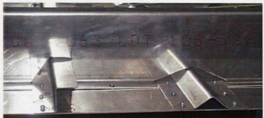
Figure 9 Frame and Stringer Arrangement for Stylised Fuselage Panel
