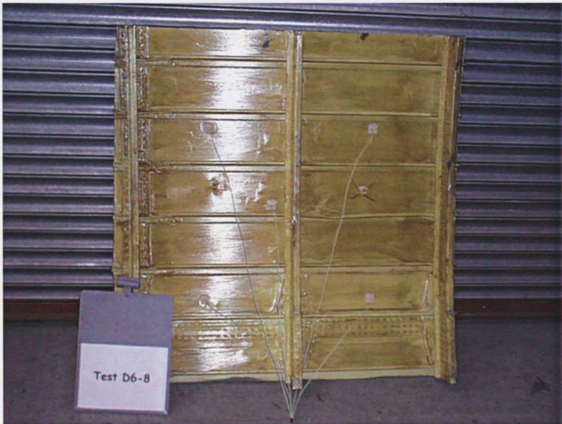
Figure 36 Test D6-8 Fuselage Panel Coated with Corrosion Inhibitors
