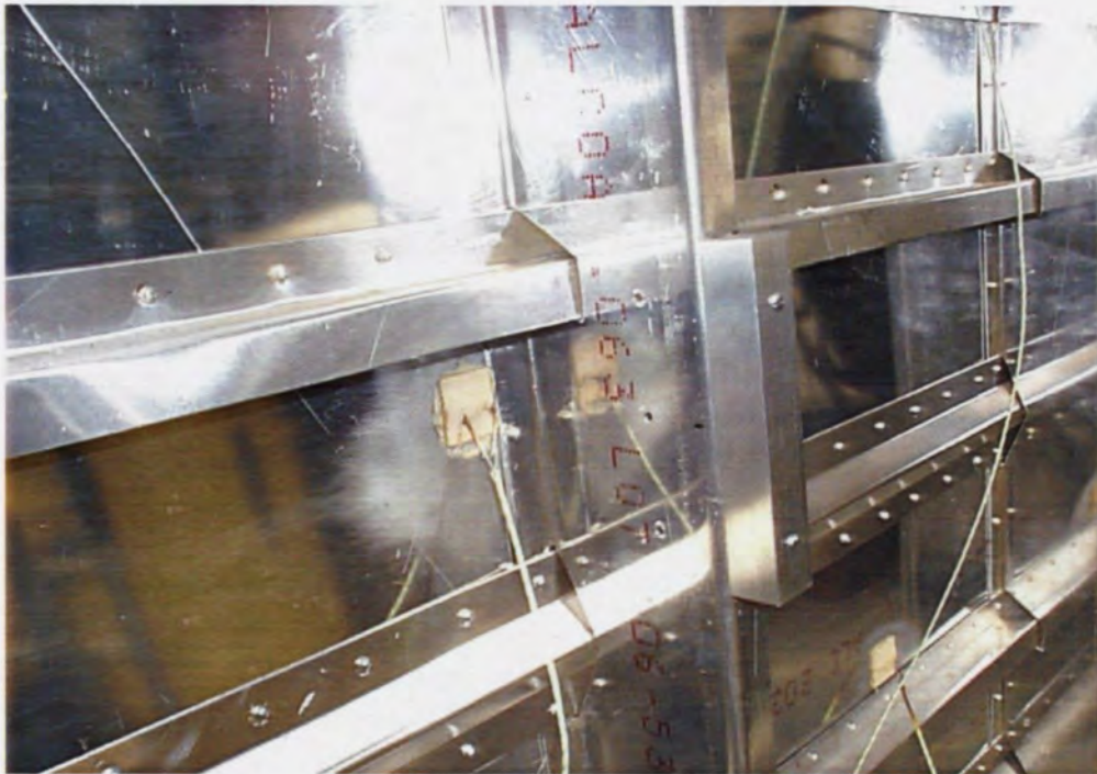
Figure 27 Simulated Clamp Block on Fuselage Frame
