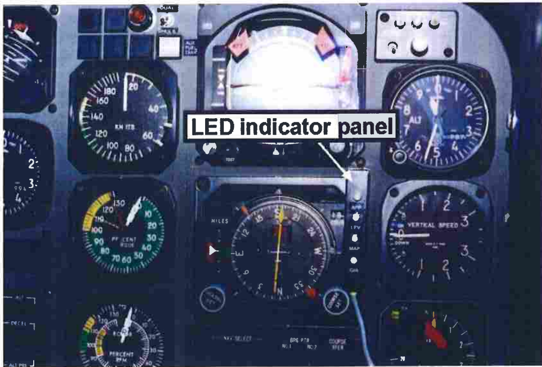
Figure 13 Cockpit LED Indicators
