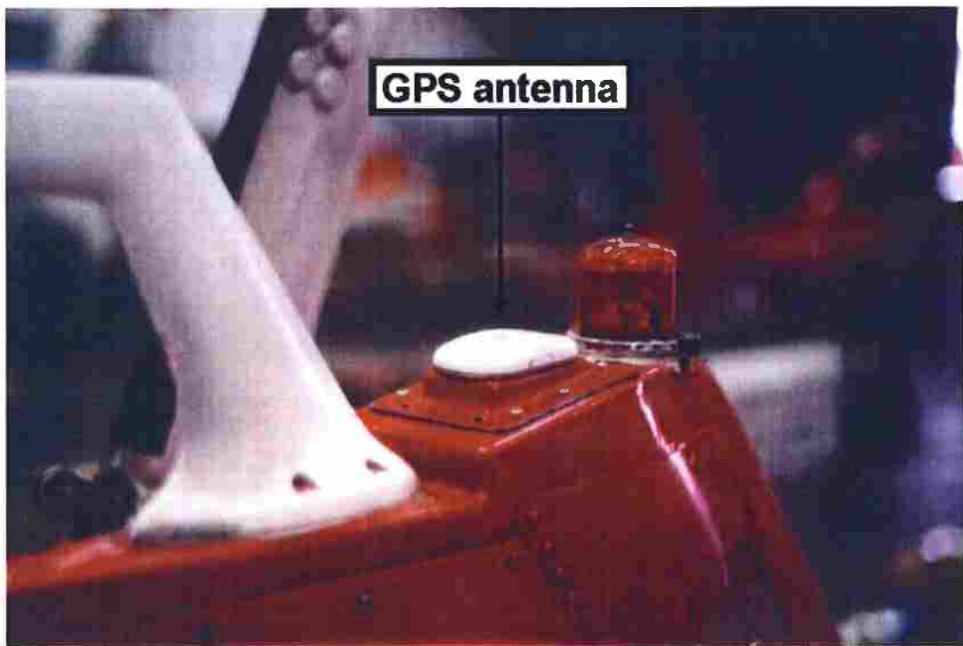
Figure 10 GPS Antenna Installation
