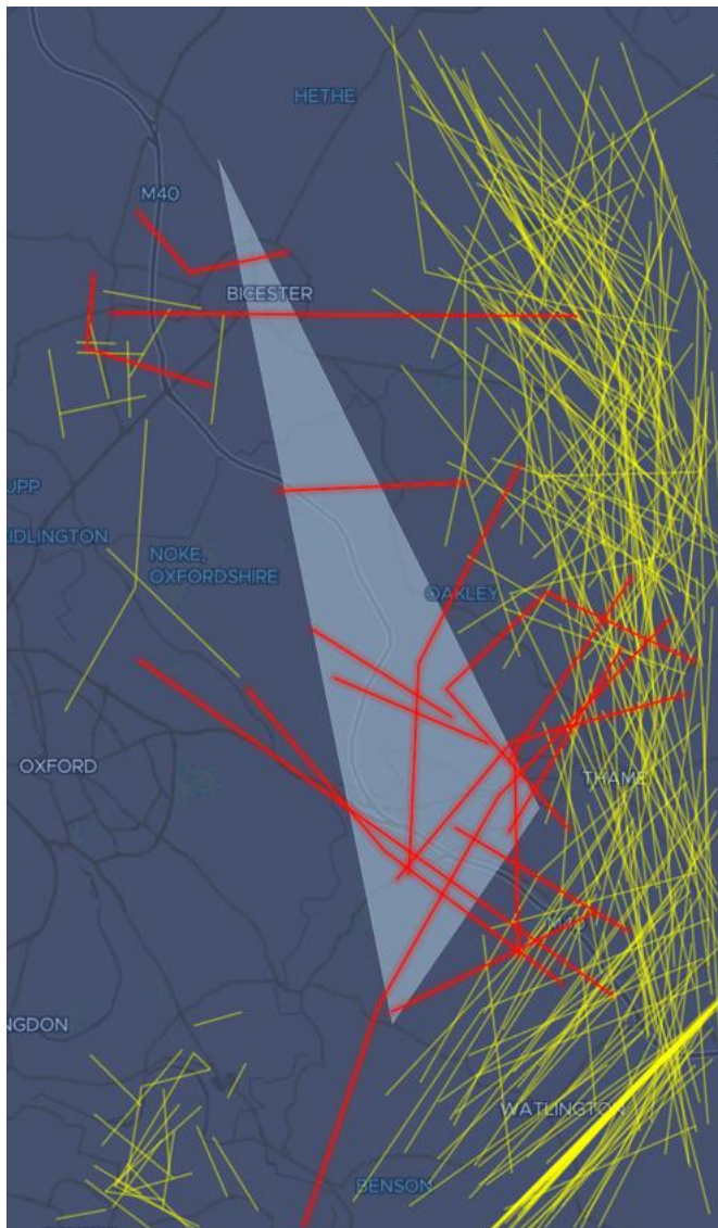
Figure 15: Daventry CTA 6 - Commercial Aircraft Tracks between FL65-FL75 (clipped to altitude) (1 January – 31 December 2019), from the CAA's Airspace Analyser Tool.
