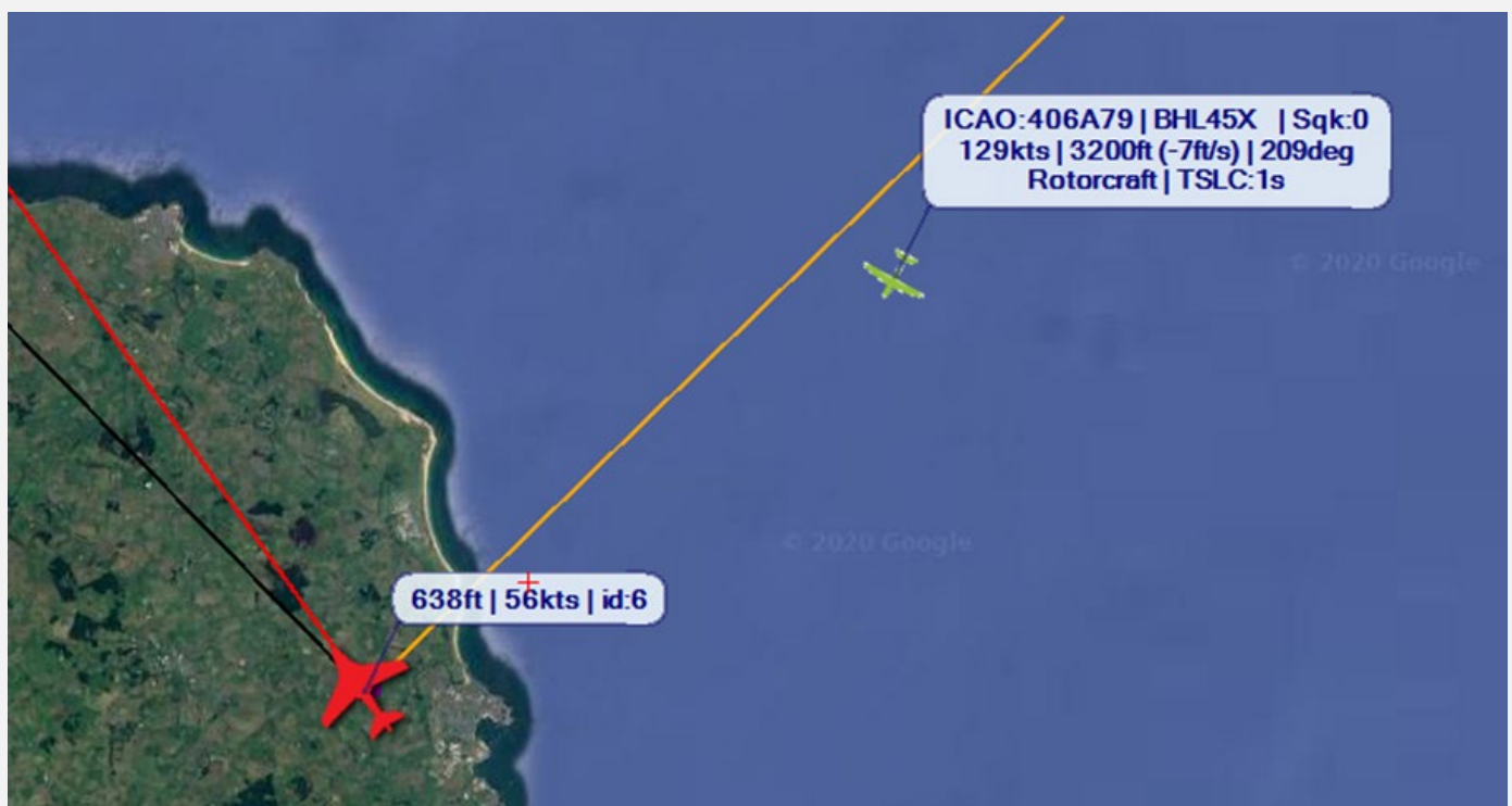
Example of Flylogix remote pilot detecting another aircraft (green icon) visible over ADS-B
