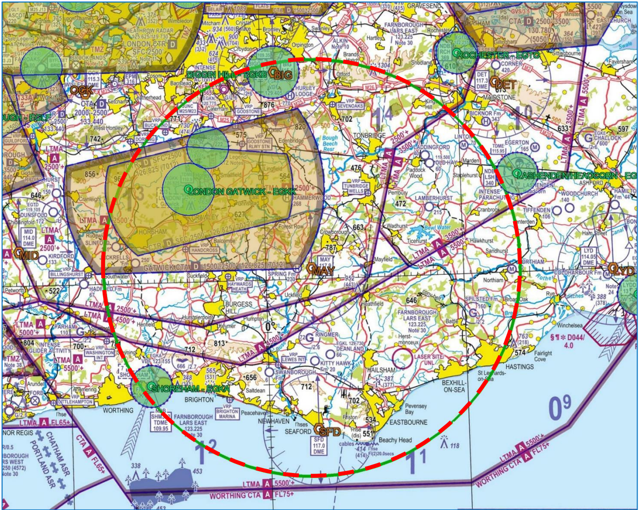
Chart 1 – Serial A1 20nm Anti-Clockwise Orbit at 4,000ft AMSL To be flown on the Gatwick QNH
