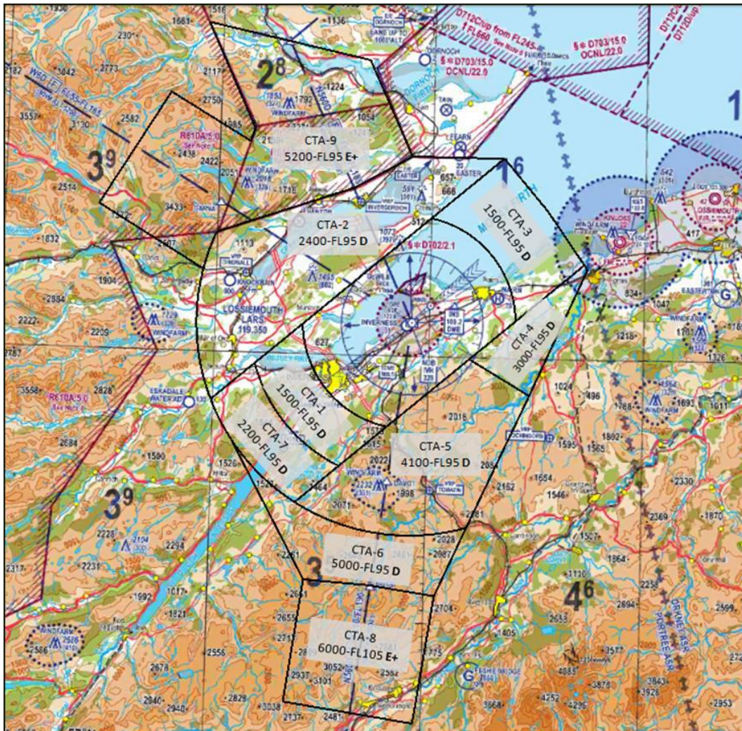
Figure 5 Proposed Inverness Class D and E+TMZ CAS – Proposal 2014 UK Civil Aviation Authority (CAA) / NATS Digital Data. VFR Chart Scotland, 500,000, June 2013
