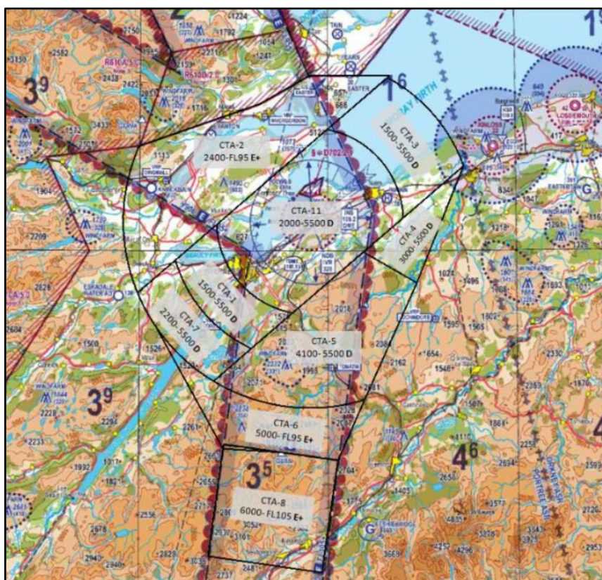
Figure 10 - Proposed Inverness Airport Class D (Ceiling 5,500ft) and E+TMZ CTAs UK Civil Aviation Authority (CAA) / NATS Digital Data. VFR Chart Scotland, 500,000, June 2013
