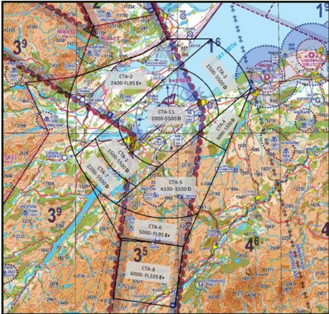
Figure 2 - Geographic extent of the Inverness Control Zone (CTR) and Control Areas (CTA) UK Civil Aviation Authority (CAA) / NATS Digital Data. VFR Chart Scotland, 500,000, June 2013
