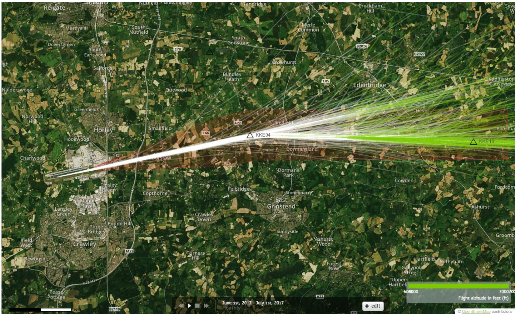
Green plots show the points at which an aircraft was between 6000 and 7000ft altitude.
