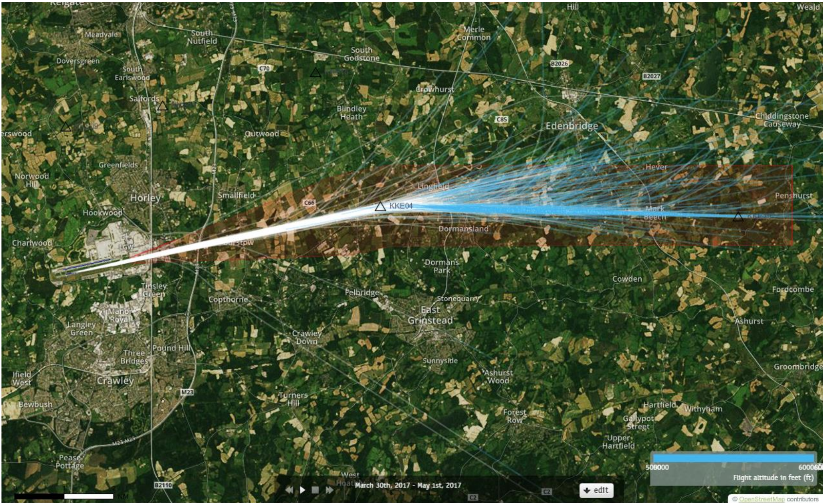
Blue plots show the points at which an aircraft was between 5000 and 6000ft altitude.
