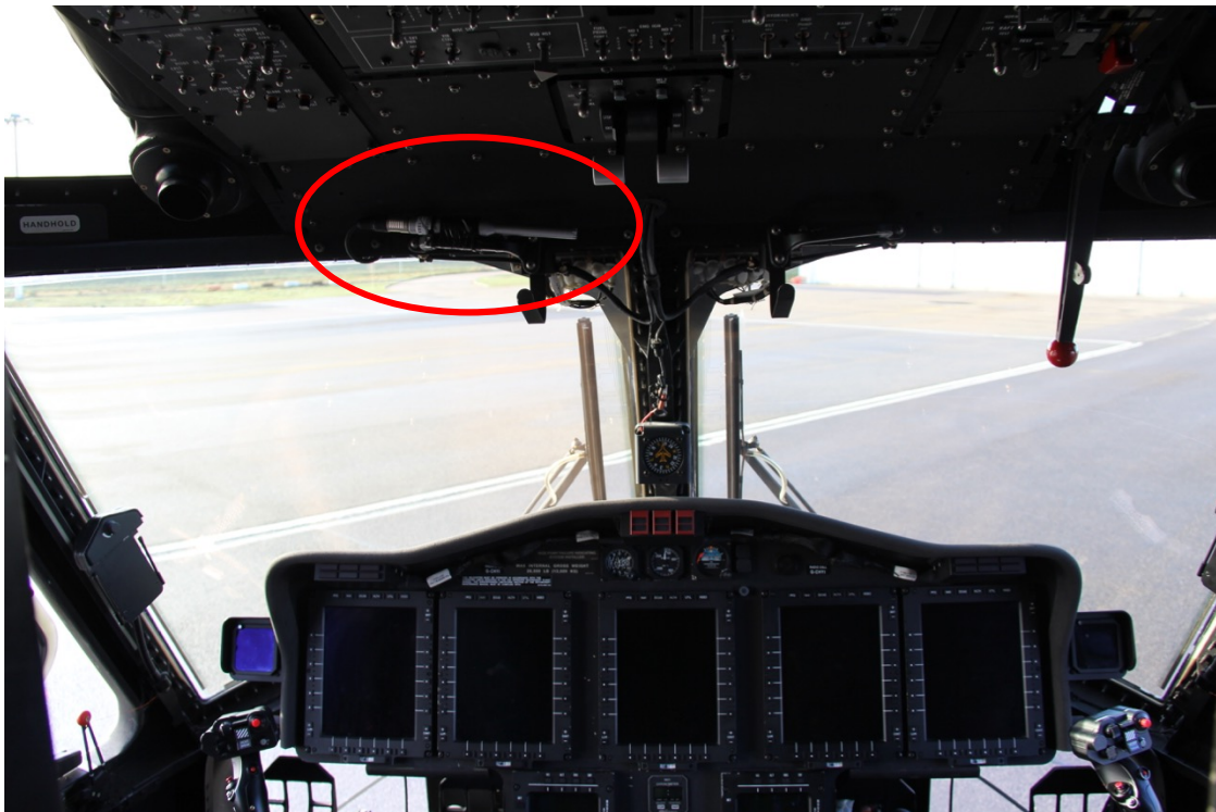
Figure 6.4 – Microphone (circled) location in flight
