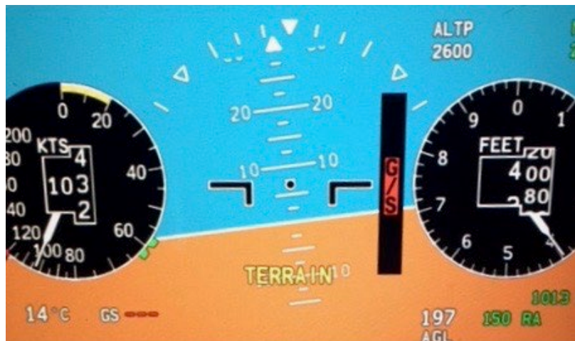
Figure 4.7 – Terrain Caution Expanded
