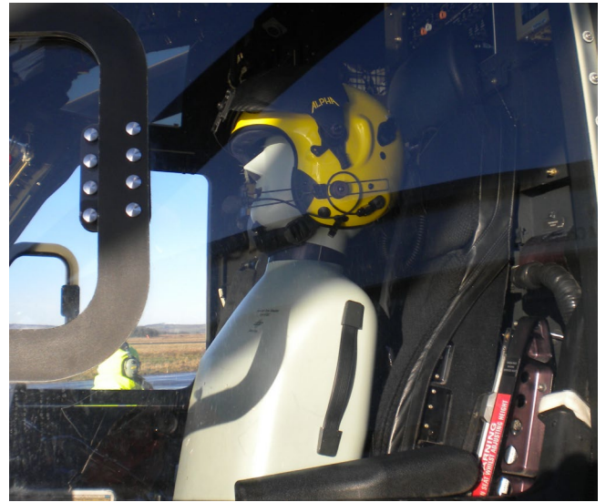
Figures 8.7 and 8.8 – HATS installed in cockpit with ALPHA Eagle helmet
