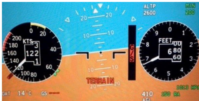
Figure 4.8 Terrain Warning Expanded
