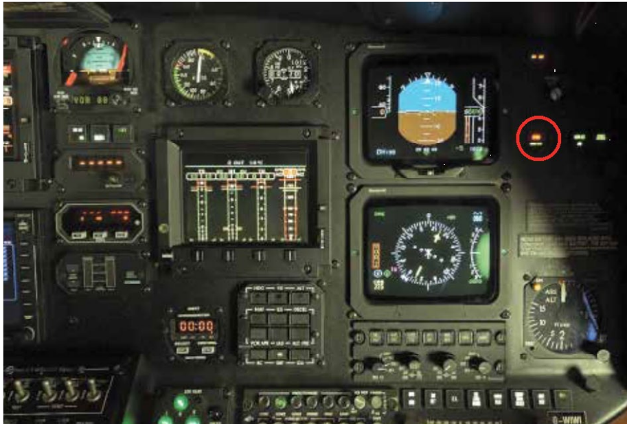
Figure A2.3 – RH instrument panel of G-WIWI showing GPWS visual alert (amber – circled red) from (Air Accidents Investigation Branch, 2014a)
