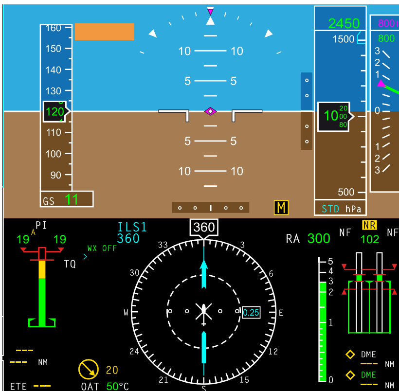
Figure 4.4 – Position and text of amber TAWS Caution messages on PFD
