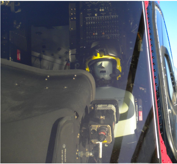
Figures 8.7 and 8.8 – HATS installed in cockpit with ALPHA Eagle helmet
