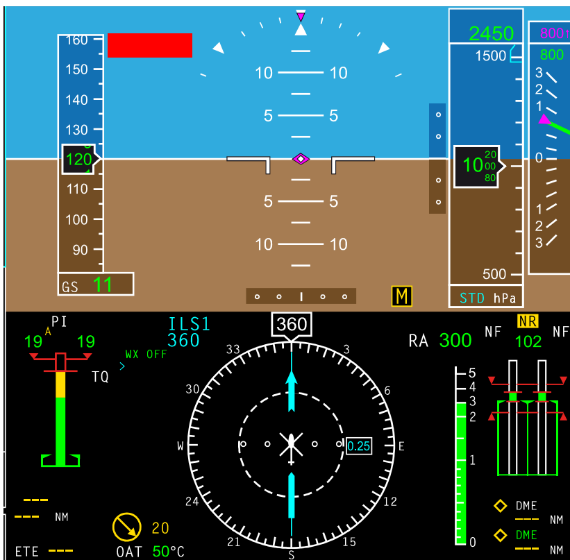
Figure 4.3 – Position and text of red TAWS Warning messages on PFD
