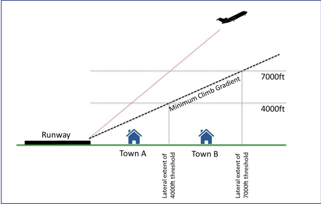
Figure 2.2: Illustration of an increased minimum climb gradient to lessen noise impacts through greater height over the ground
