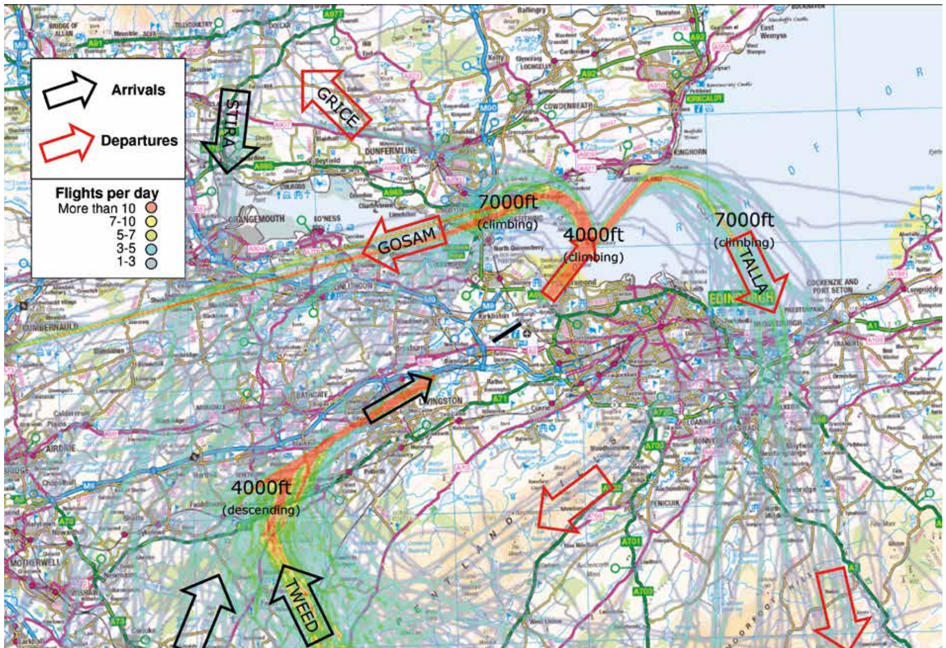
Figure 4: Current flight paths with typical altitudes, runway 06 easterly operations
