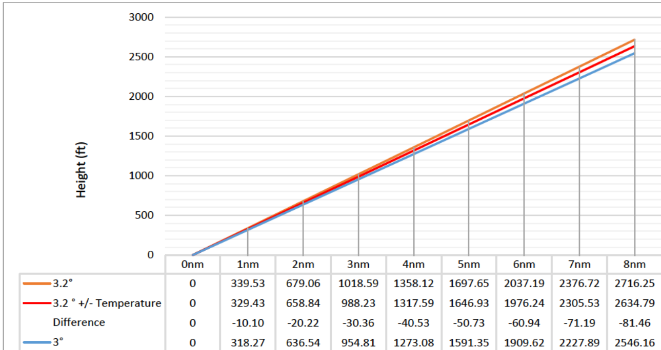
Figure 34: Effect of an average temperature of 6.5°C air temperature on a 3.2° Baro-VNAV approach
