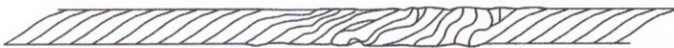
Fig 9 – Example of Nyvin wire, straightened after "knuckling", with the insulation removed, to show displacement of wire strands.
