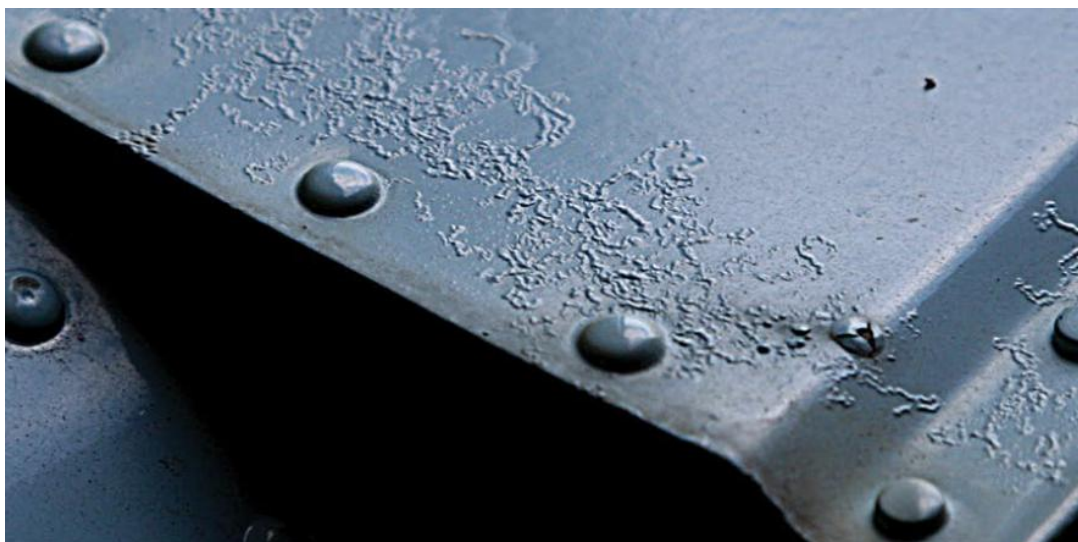
Photograph 6. Filiform corrosion spreading from scribe on painted aluminium after complete accelerated corrosion testing 3
