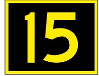
Runway Location Sign
