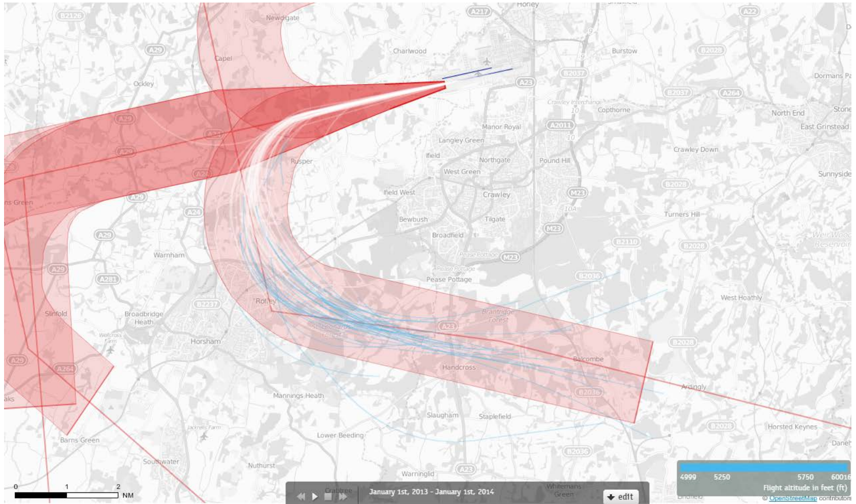
Blue plots show the points at which an aircraft was between 5000 and 6000ft altitude.
