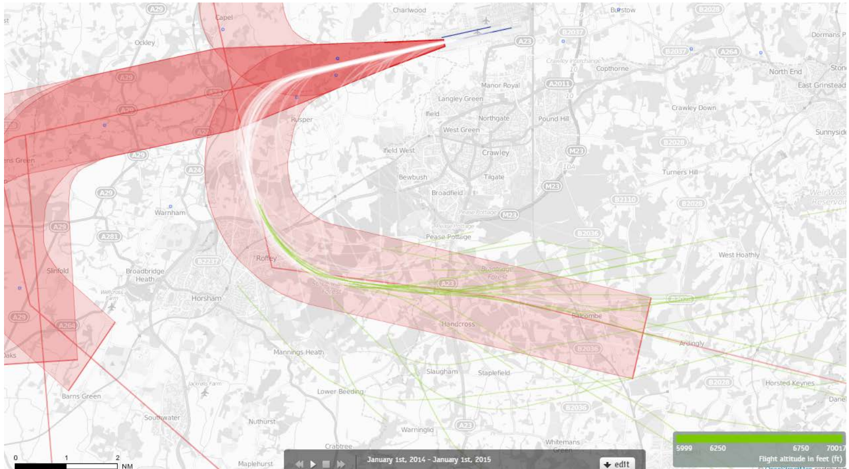
Green plots show the points at which an aircraft was between 6000 and 7000ft altitude.
