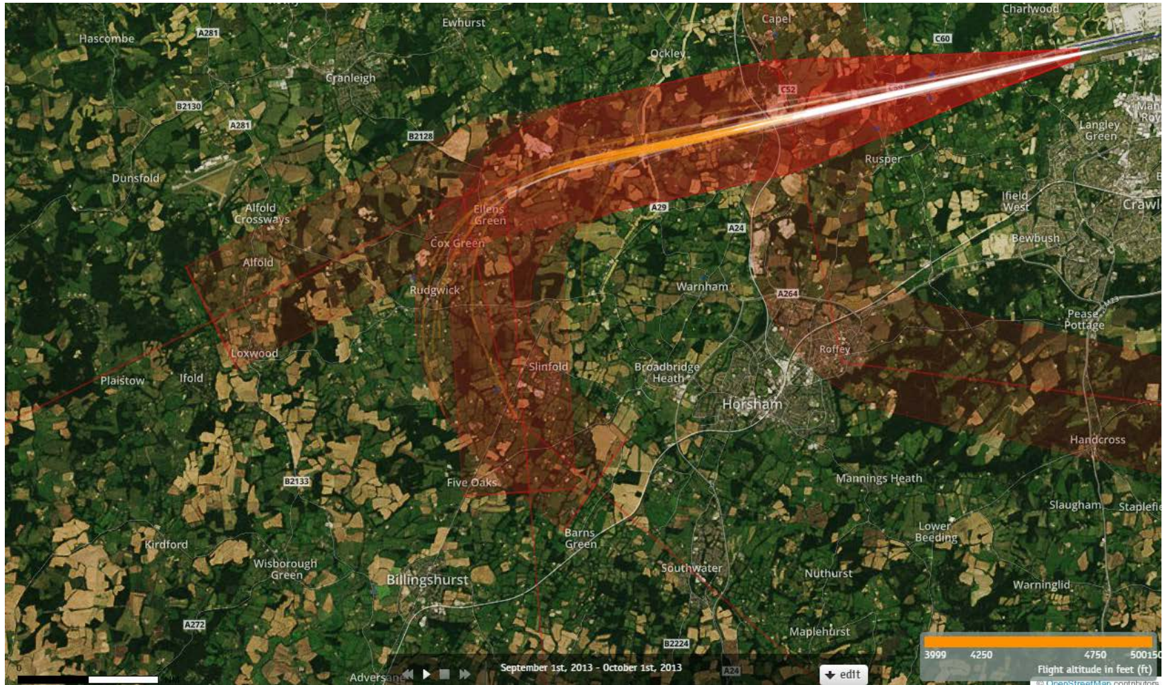
Orange plots show the points at which an aircraft was between 4000 and 5000ft altitude.
