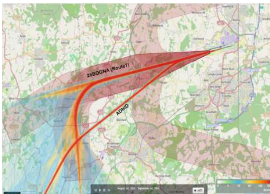
Figure 9 – Departures on the Route 7 SIDs also showing the departures on the ADNID trial on 8 August 2014
