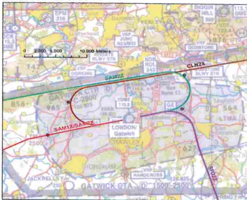
Figure 2.1: P-RNAV SID centrelines and speed trial points.
