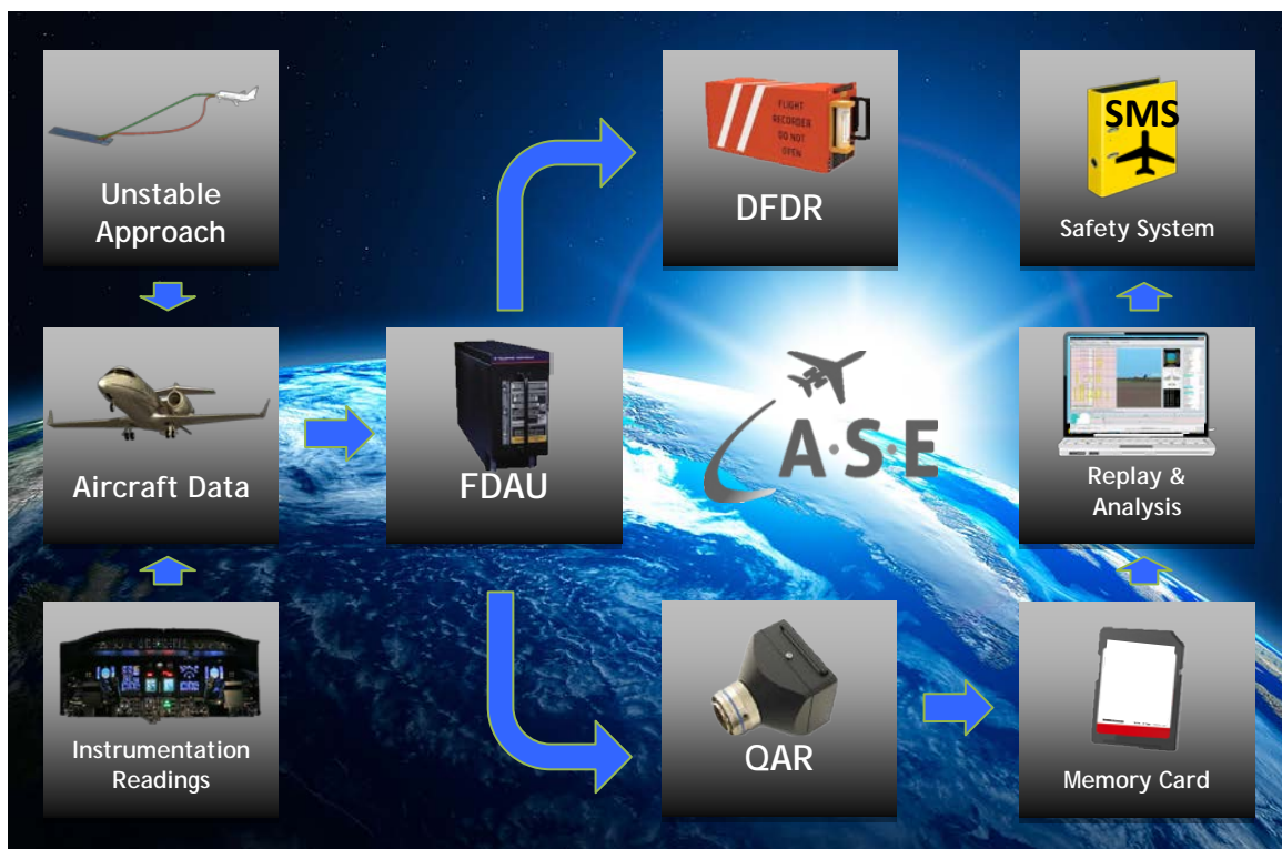
Diagram 4: (FDM System Flow Diagram)
