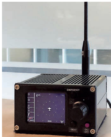
How LPAT looks in operation. It's designed to be 'carry on' equipment rather than being panel-mounted, reducing both certification requirements and installation costs. The Trig version interacts with another screen.
