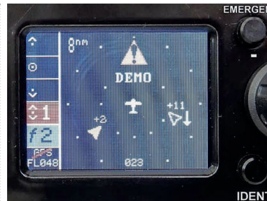
How LPAT looks in operation. It's designed to be 'carry on' equipment rather than being panel-mounted, reducing both certification requirements and installation costs. The Trig version interacts with another screen.
