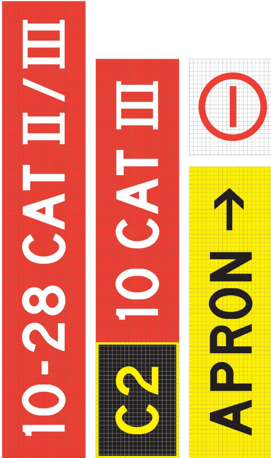
Figure 7A.8 Sign face size proportions and layout
