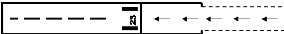
Figure 3H.1 Starter extension and pre-threshold markings
