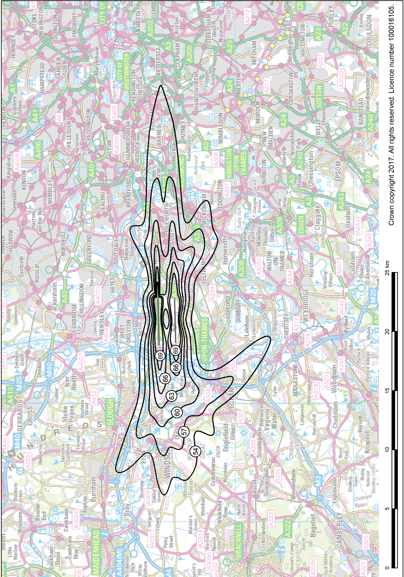
Figure 5 Heathrow 2016 Leveing 54-69 dBA contours
