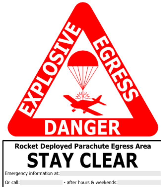
Figure X2 - Sample label with danger placard. Danger placard to be dimensioned in as defined in Figure X1.
