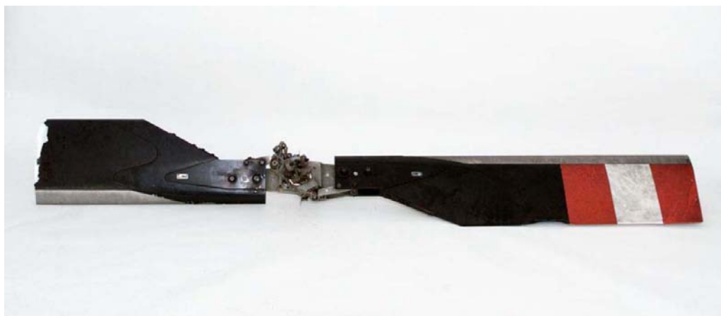
Figure 3-1: TR Blade Failure
