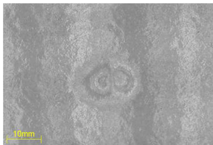
Figure 12 15 J, 20 mm impact on 17 ply painted laminate
