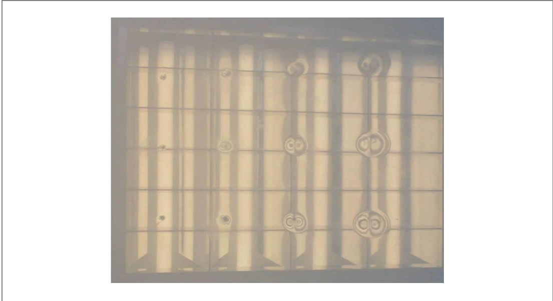
Figure 6 Surface flaws producing distorted reflections
