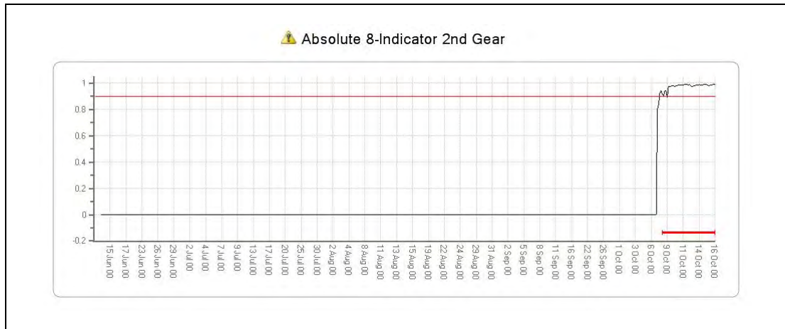
Figure 4-2 The '8IA' model PA output for the cracked MGB bevel pinion fault case
