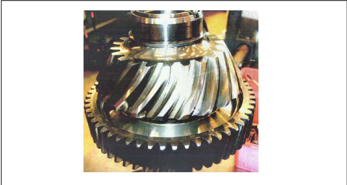
Figure 2-7 Picture of the bevel pinion with a large visible crack
