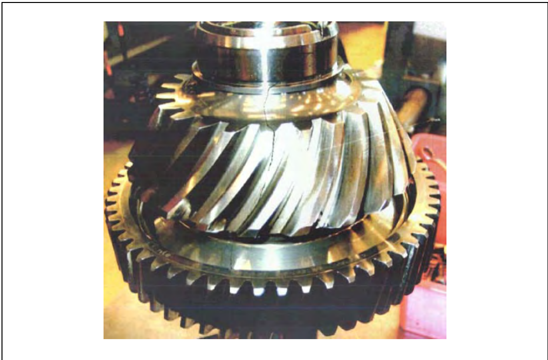
Figure 7-1 Picture of the bevel pinion with a large visible crack
