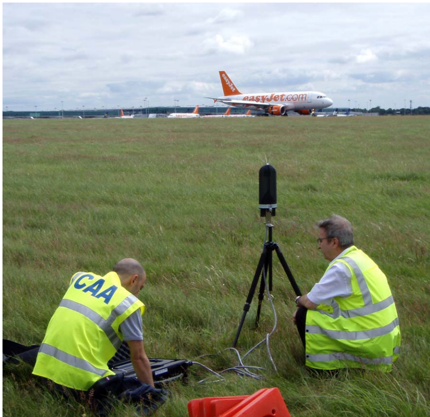
Figure 2 Set up of an airside noise monitor at Stansted
