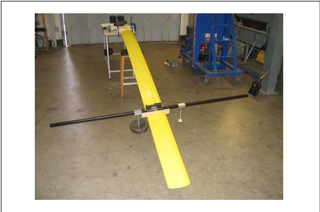
Figure 9 Arrangement of the experimental measurements of EA position and torsional stiffness of the blade
