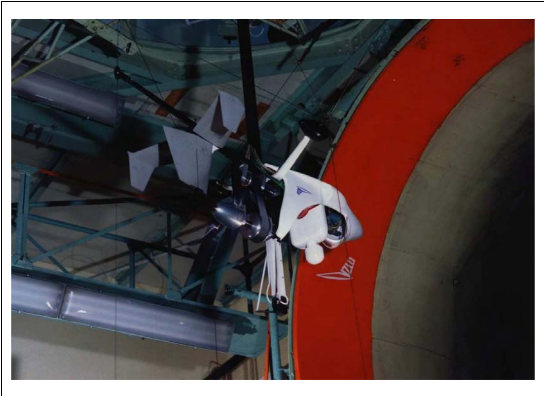
Figure 3.4 b) VPM M14 Model in VZLU Wind Tunnel (Rear View)
