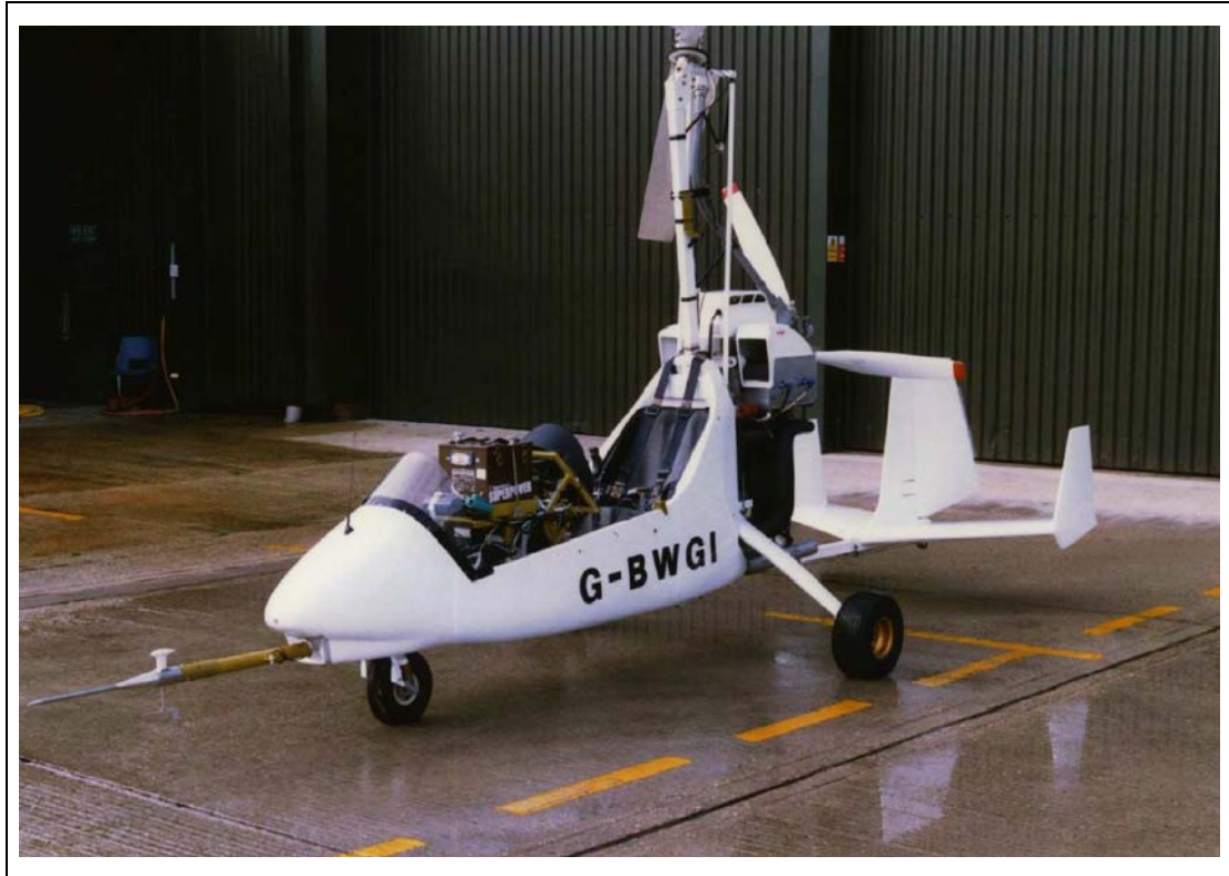
Figure 5.4 a) Flight Test Instrumentation for VPM M16 G-BWGI Flight Trials (G-BWGI in Modified Form for Flight Trials)
