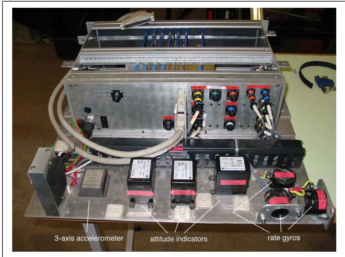
Figure 5.5 c) G-UNIV Flight Test Instrumentation (Sensors On-board Main Instrumentation Pallet)
