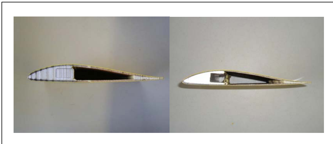
Figure 6 Internal structure of the rotor blade from Montgomery-Parsons research Gyroplane. Left section comes from the root of the blade while the right one was located close to the tip of the rotor blade
