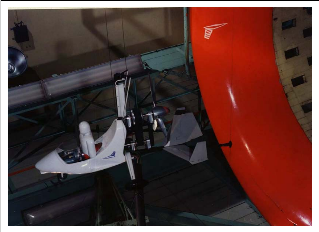
Figure 3.4 a) VPM M14 Model in VZLU Wind Tunnel (Front View)
