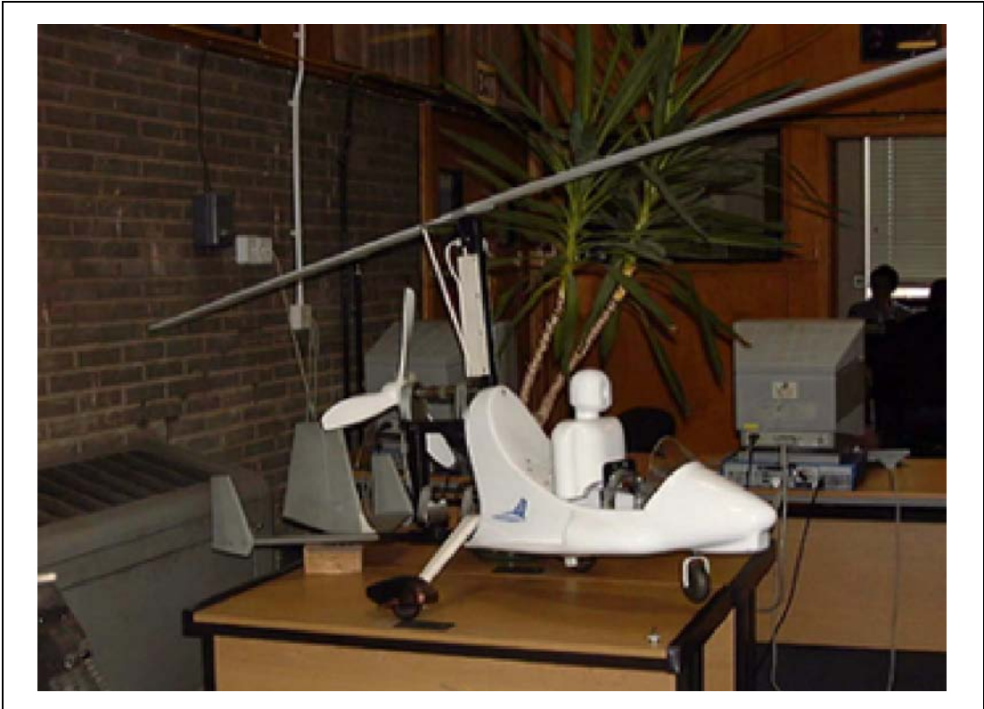
Figure 3.2 One Third Scale Wind Tunnel Model of a VPM M14 Gyroplane
