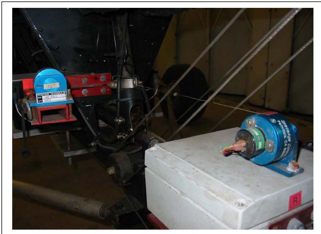
Figure 5.5 d) G-UNIV Flight Test Instrumentation (Displacement Transducers for Measurement of Stick Position)
