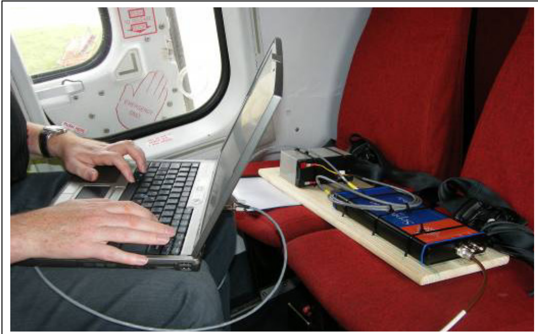
Figure 5.2 Airborne trials installation located in forward passenger seats with connection to aircraft GPS antenna
