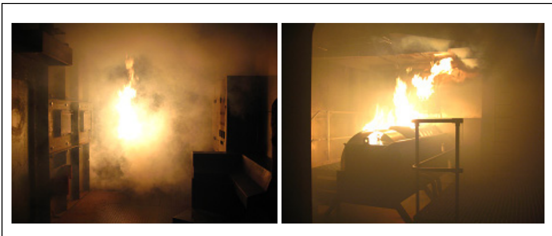
Figure 27 Machinery Control Room Fire Rig and Engine Fire Rig on Lower Deck
