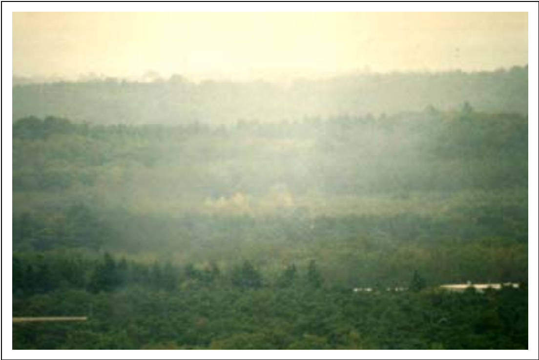
Figure 13d Variation of plume density using 50%/50% glycerol/water solution – test point 12, one pressure-jet, 60 seconds duration
