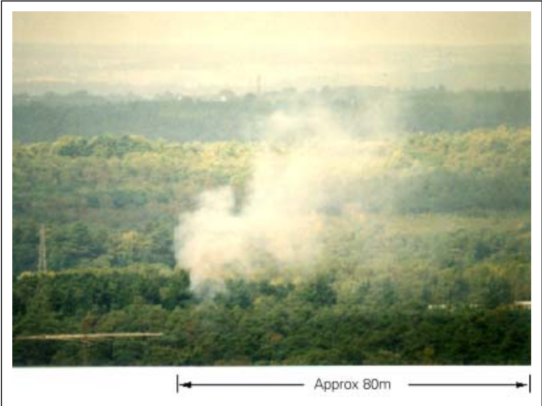
Figure 14a Variation of density using theatrical smoke oil – test point 18, four pressure-jet atomisers, 60 seconds duration
