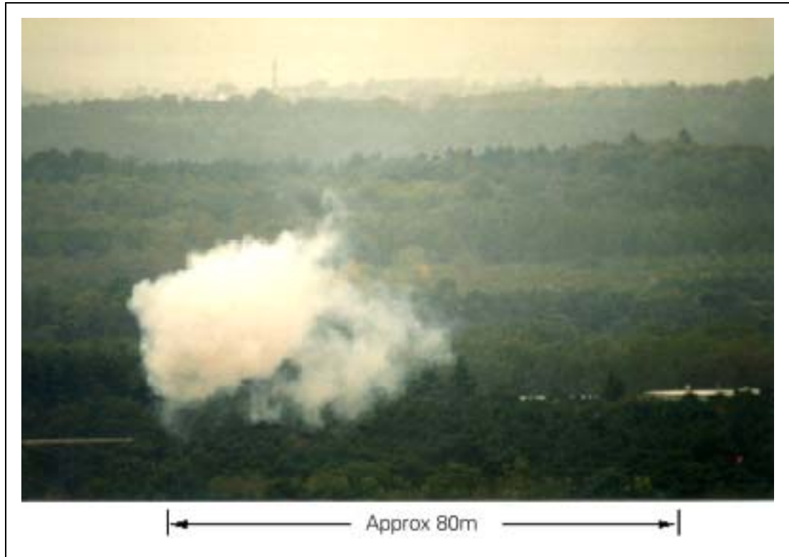
Figure 10a Variation of plume density with time using glycerol/water 50%/50% concentration – test point 9, plume density, four pressure jet atomisers, 30 seconds duration
