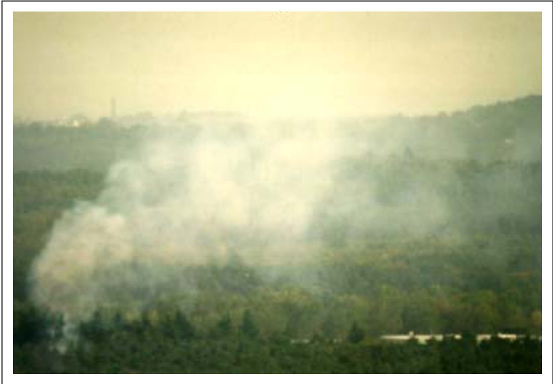
Figure 17a Comparison of different flow rates for diesel using air-blast atomisers – test point 5, two air-blast atomisers at 14.5 bar, 60 seconds duration
