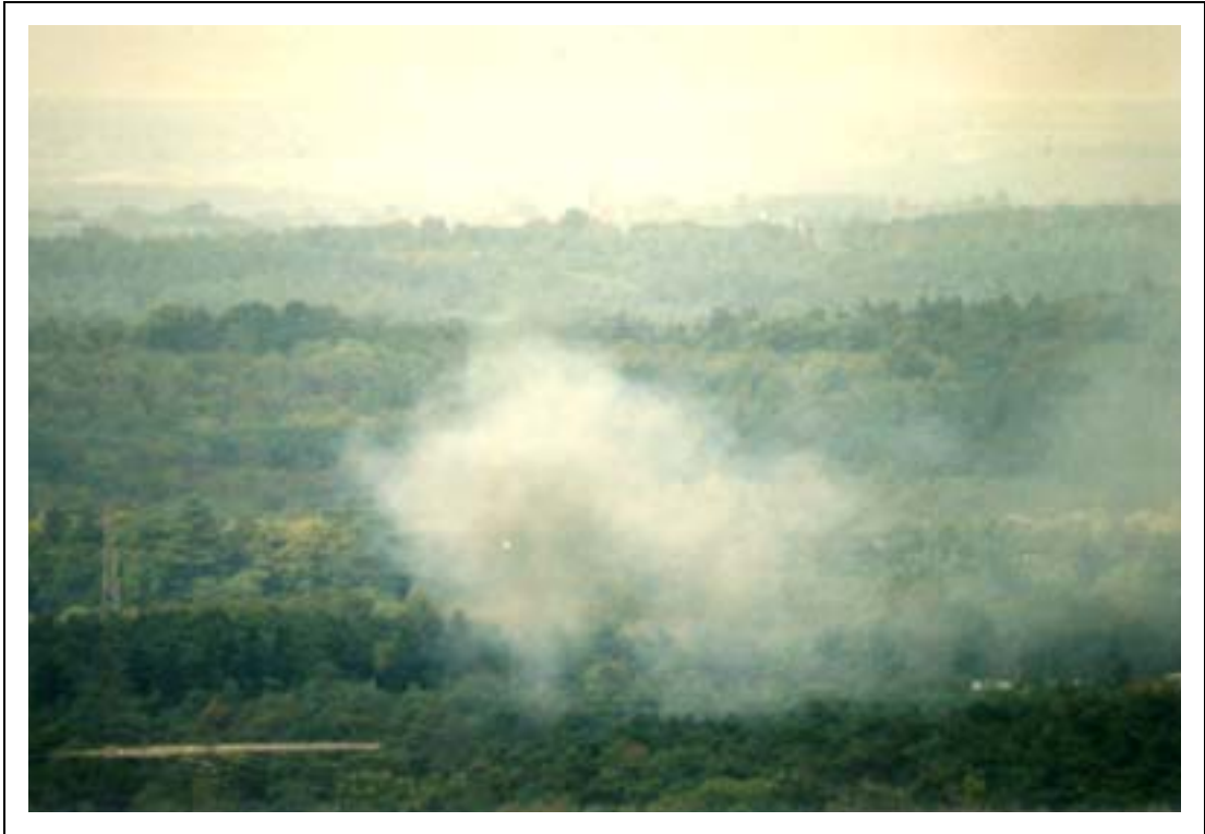
Figure 16a Comparison of different flow rates for theatrical smoke oil using air-blast atomisers – test point 26, two air-blast atomisers at 14.5 bar , 60 seconds duration
