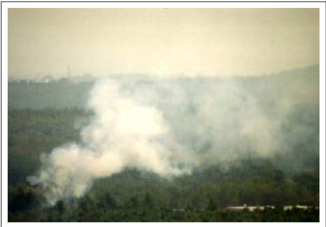
Figure 9b Comparison of air-blast and pressure-jet atomisers, diesel agent – test point 3, two pressure-jet atomisers, 60 seconds duration
