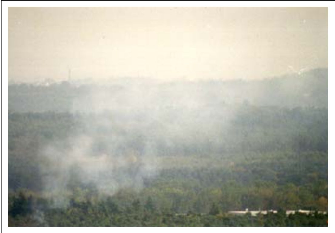
Figure 8d Variation in plume density using diesel agent – test point 4, one pressure-jet atomiser, 30 seconds duration
