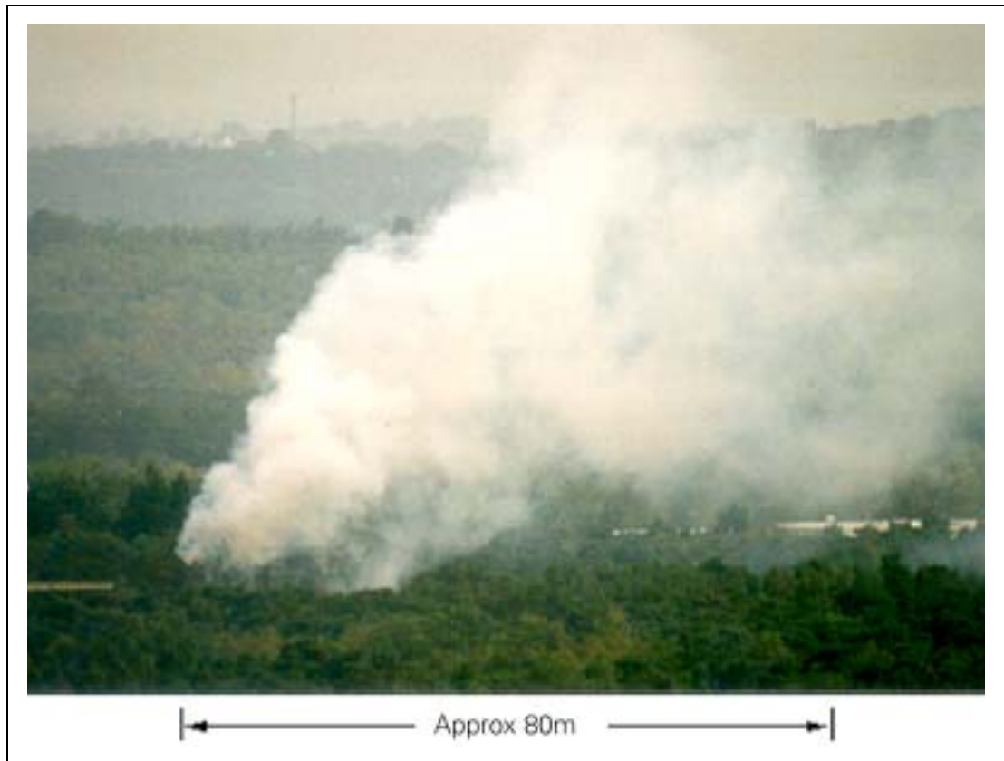
Figure 8a Variation in plume density using diesel agent – test point 1, four pressure-jet atomisers, 20 seconds duration
