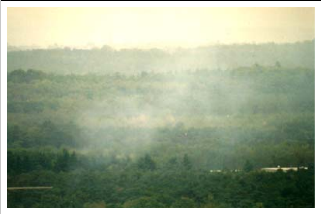
Figure 13c Variation of plume density using 50%/50% glycerol/water solution – test point 11, two pressure-jets, 60 seconds duration
