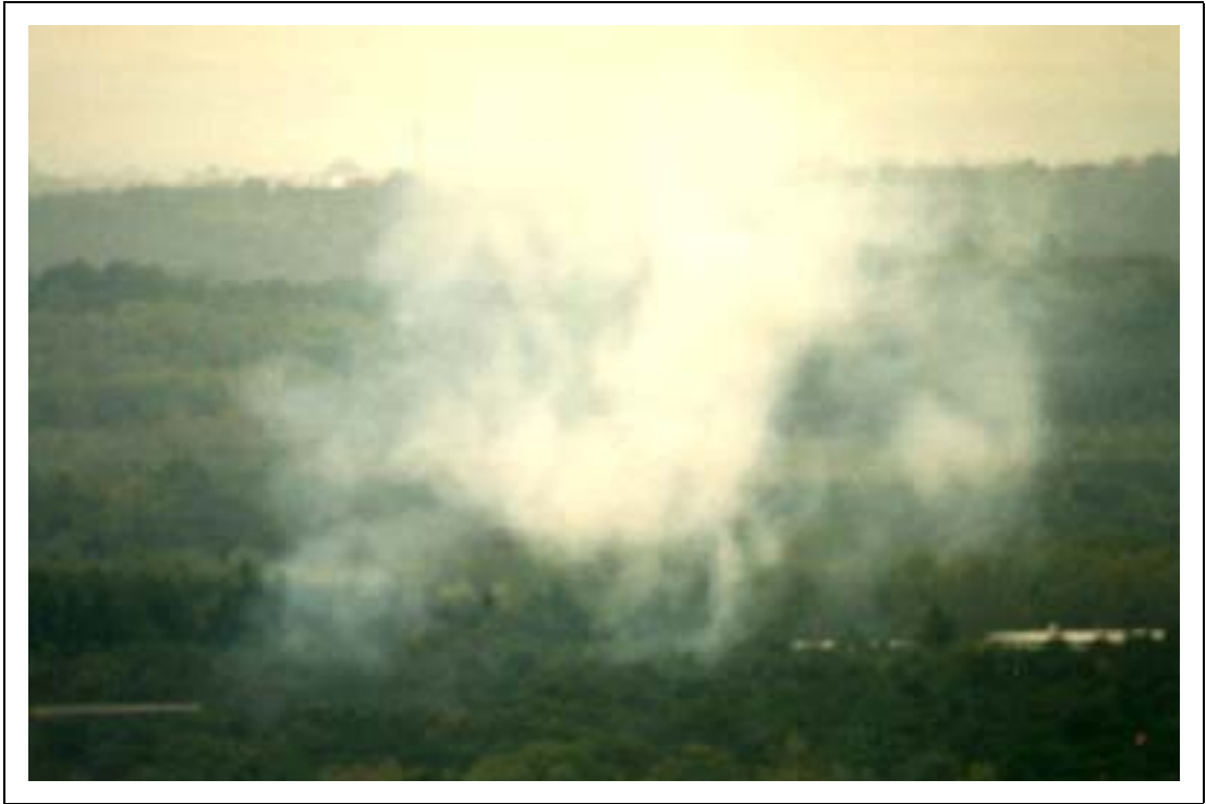
Figure 13a Variation of plume density using 50%/50% glycerol/water solution – test point 9, four pressure-jets, 60 seconds duration
