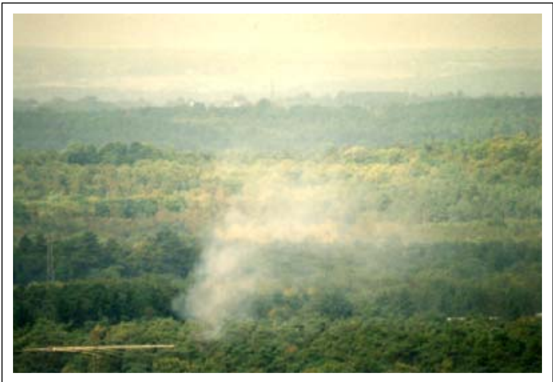
Figure 16b Comparison of different flow rates for theatrical smoke oil using air-blast atomisers – test point 22, two air-blast atomisers at 6.8 bar, 60 seconds duration
