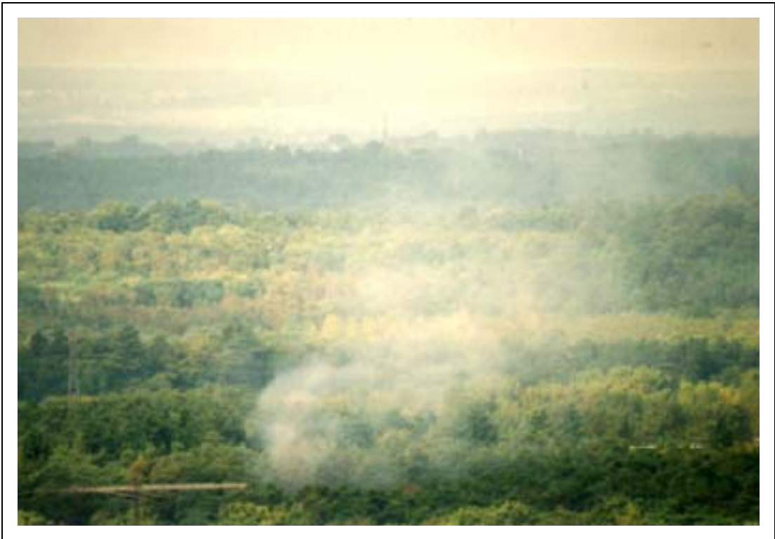
Figure 14b Variation of density using theatrical smoke oil – test point 19, three pressure-jet atomisers, 60 seconds duration
