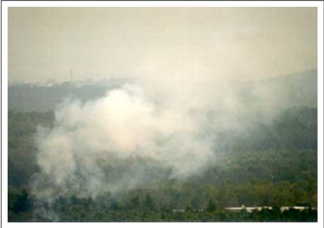
Figure 8c Variation in plume density using diesel agent – test point 3, two pressure-jet atomisers, 30 seconds duration
