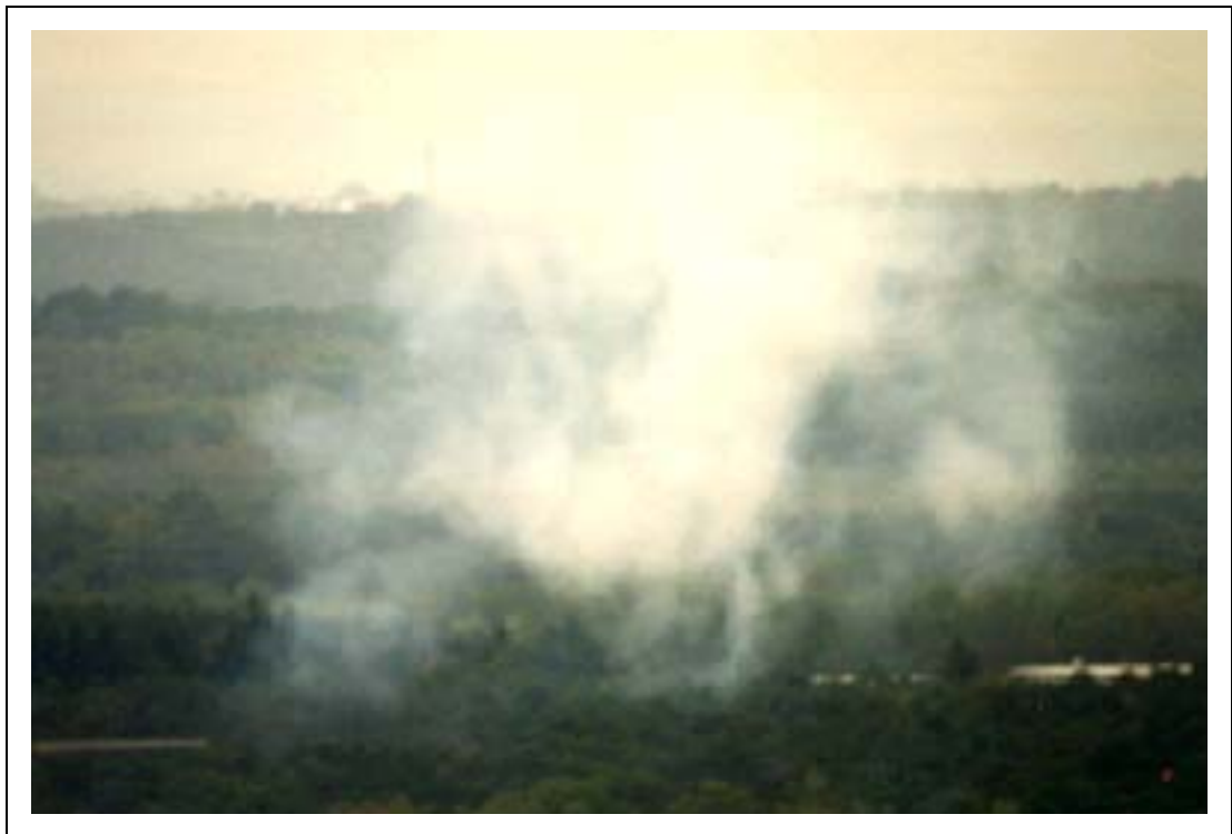
Figure 10b Variation of plume density with time using glycerol/water 50%/50% concentration – test point 9, plume density, four pressure jet atomisers, 60 seconds duration
