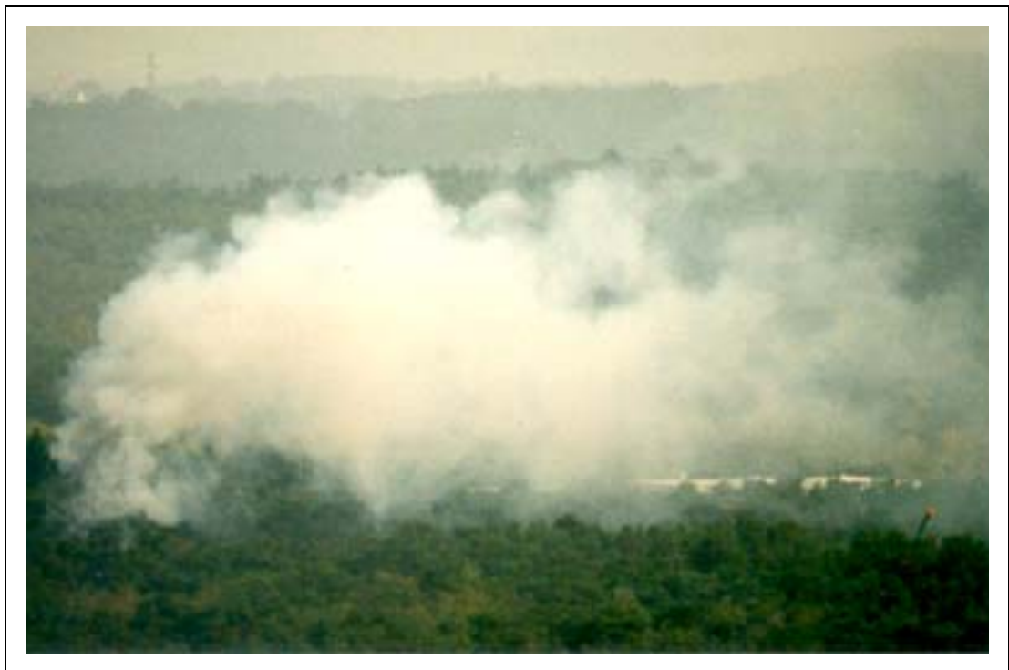
Figure 8b Variation in plume density using diesel agent – test point 2, three pressure-jet atomisers, 30 seconds duration
