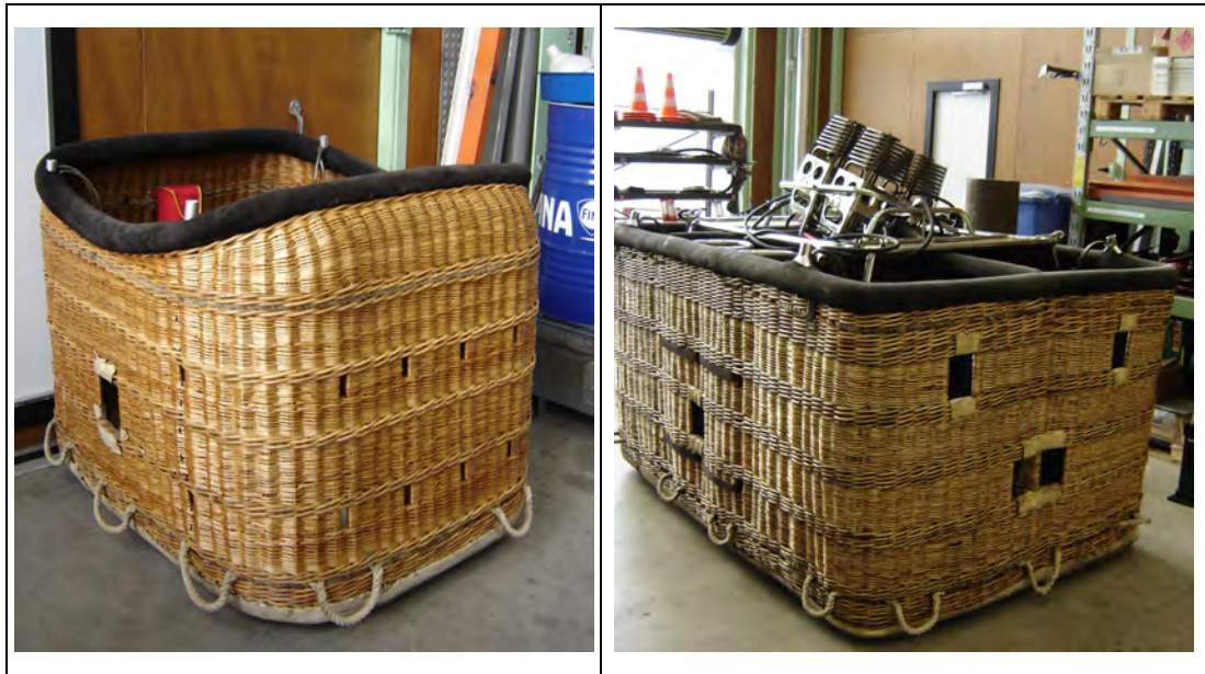
Figure 1 Baskets used to experimentally determine the force-deformation characteristics. Left: Open basket; Right: Double T-partitioned basket.
