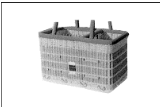
Figure 2 Single partitioned basket. The pilot and the fuel cylinders are in the small compartment separated from the passengers.
