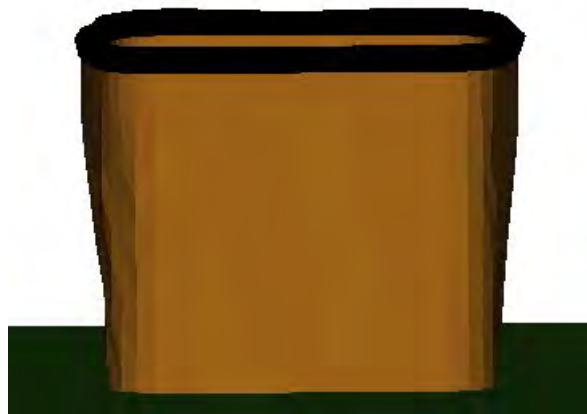
Figure 5 The flexible open basket model in deformation configuration A at maximum displacement.
