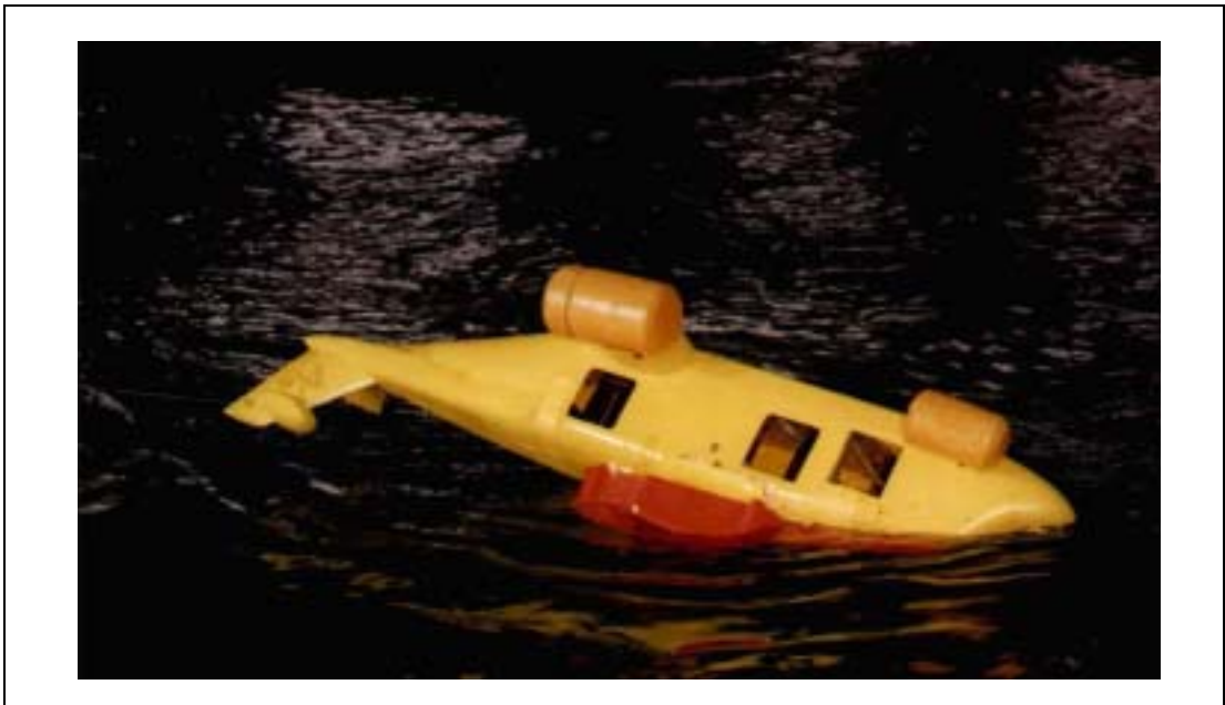
Figure 13 Model fitted with foam-filled cowling panels following capsize.
