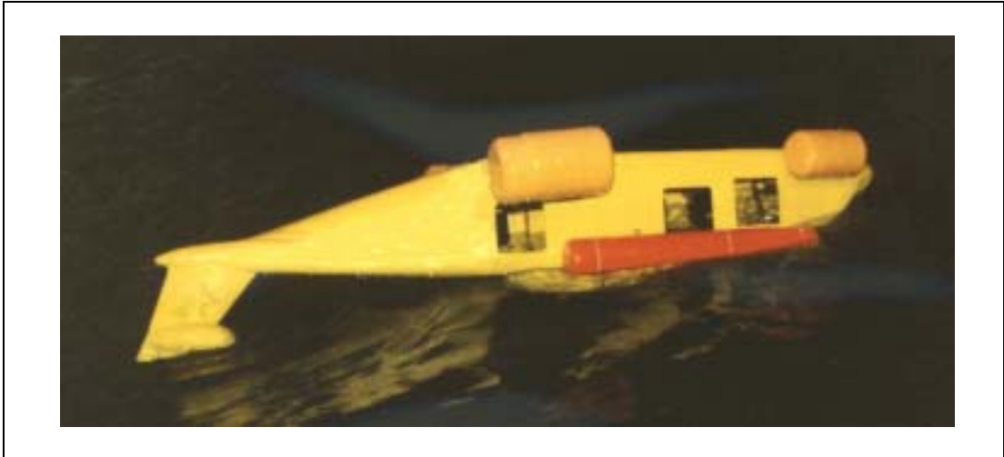
Figure 14 Model fitted with cabin wall floats following capsizes.
