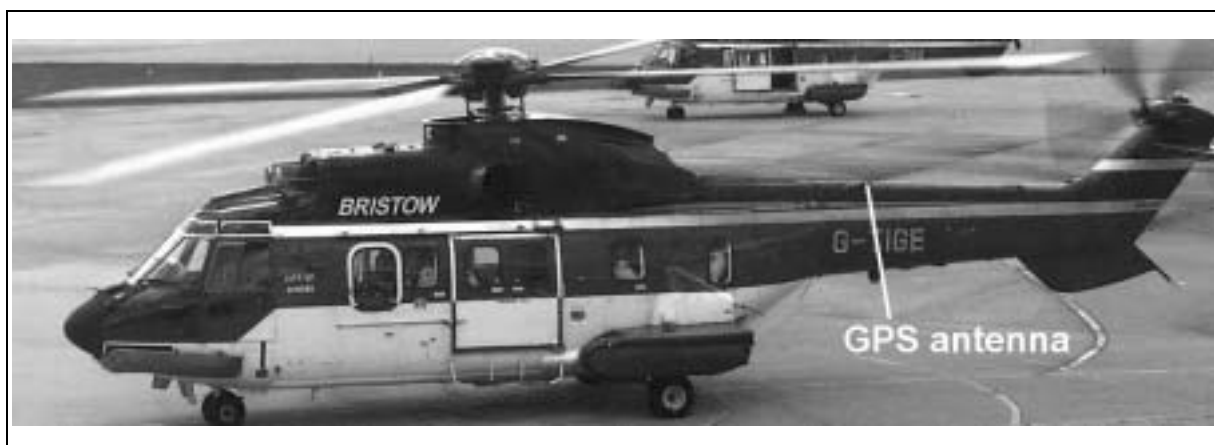
Figure 2 GPS antenna location on Super Puma G-TIGE
