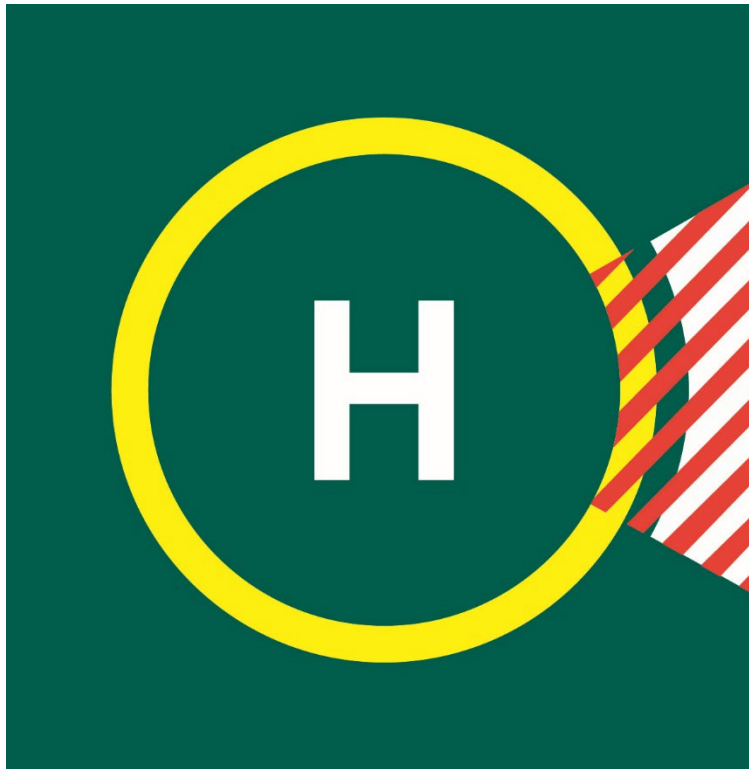
Figure 6: Example of prohibited landing heading marking
