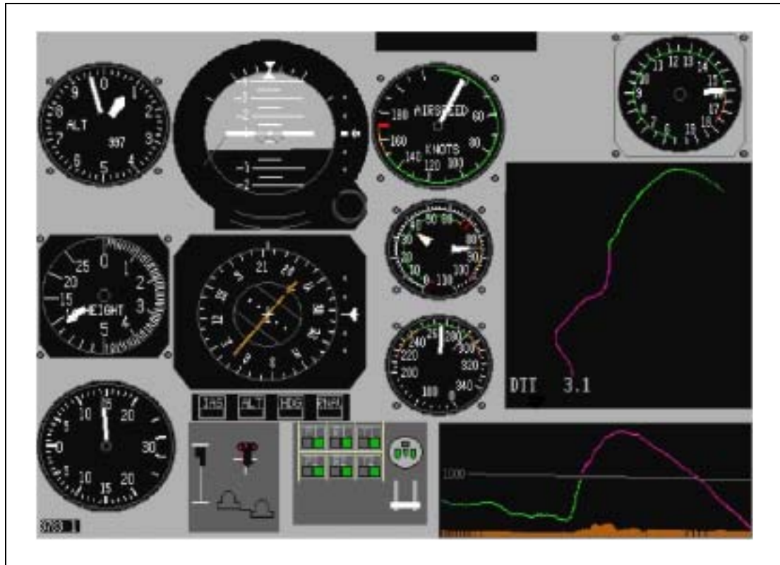
Figure 6.3 FDS View Showing Loss of Airspeed During Climb
