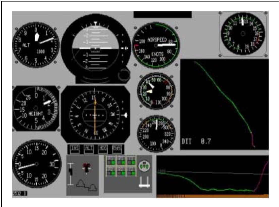
Figure 6.5 FDS View During an Airborne Radar Approach
