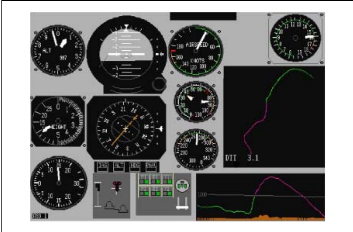
Figure 4.4 Super Puma FDS Display
