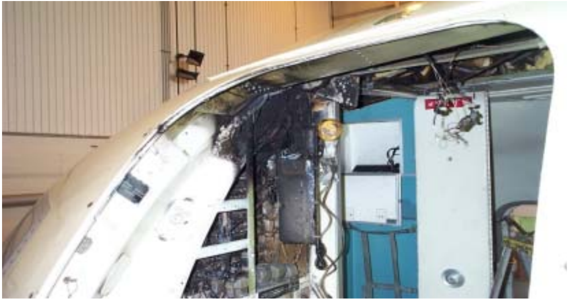
Figure 1 Fire in Bulkhead, Spread to Area Above Cabin Ceiling (Overhead)
