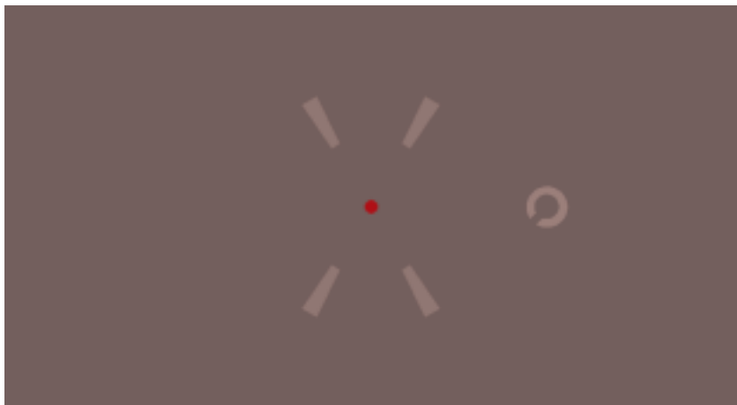
Fig.ii Screen dump of stimulus configuration employed in the CAA test. The picture shows the stimulus at +2.5^\circ eccentricity, together with central fixation target and guides
