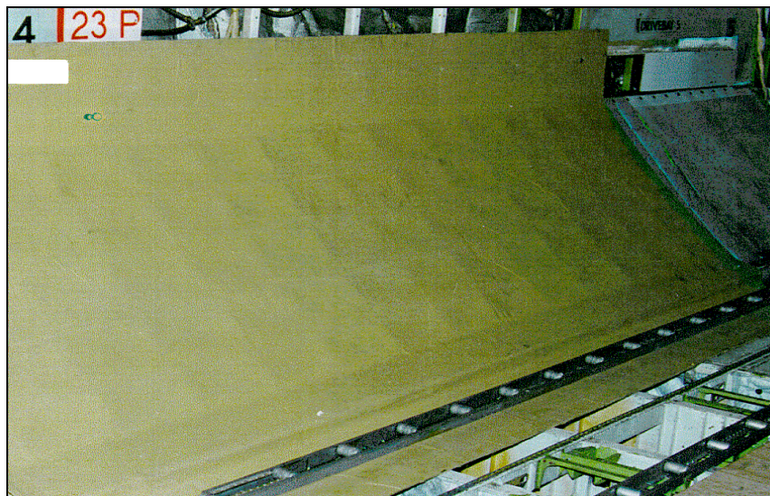
Figure 4 A hardened liner in position prior to test. It is situated in the cargo bay, placed over the frames and extending over seven bays
